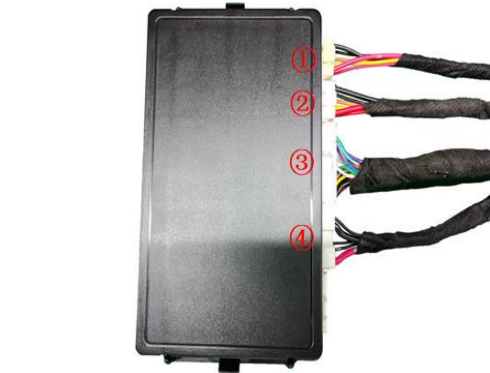
26. Insert the left and right strut wiring harnesses ① ②, lock signal harness ③, and power harness ④ into the ECU in sequence.
