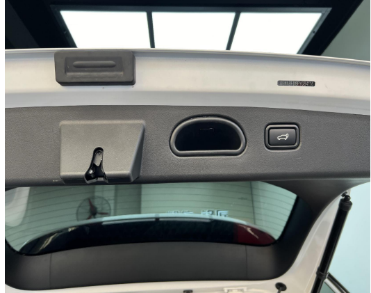
29. Install the added tailgate switch and reinstall all trim panels.
