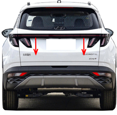
27. Press the added tailgate switch to close the tailgate once, the system completes initialization, and then test each function of the electric tailgate.
