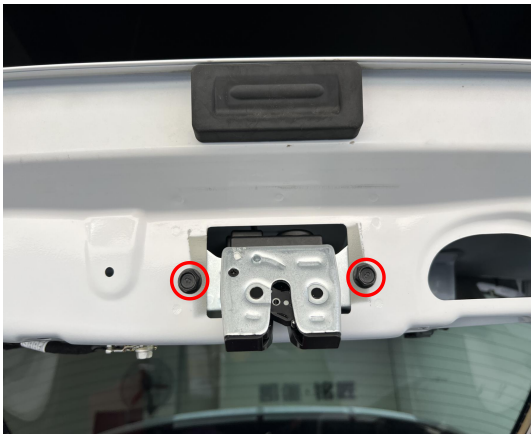
12. Remove the original latch.
