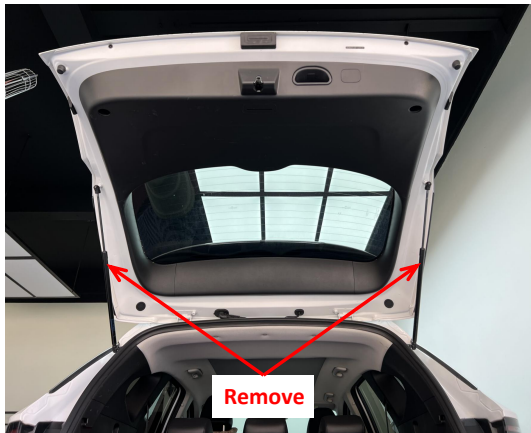
5. Remove the original gas struts.
