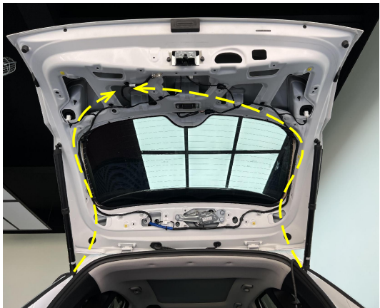
11. Route the strut wiring harnesses as indicated above.
