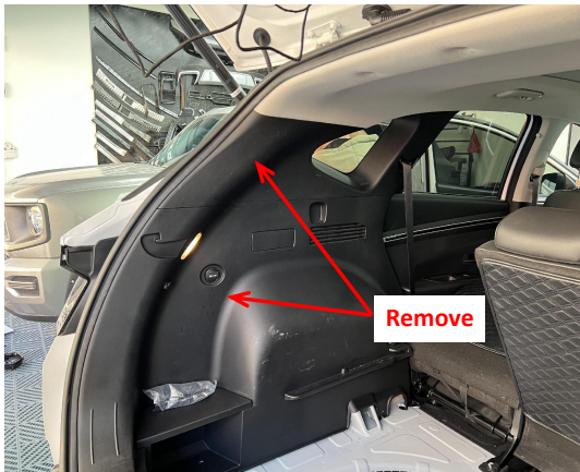
3. Remove the trim panels on the left side of the trunk.
