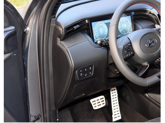
(Optional) Find an appropriate position at the driver's area, drill a \phi 21\text{mm} hole and install the added front switch.
