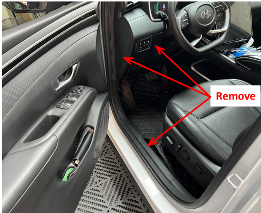
1. Remove the indicated driver's side trim panels.
