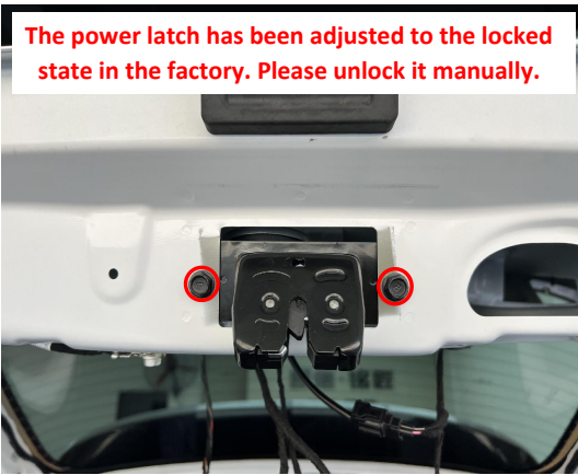
14. Install the power latch.
