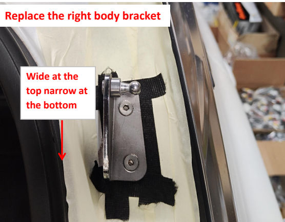
7. Replace the right body bracket and pay attention to the direction.
