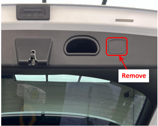
28. Remove the indicated small panel.
