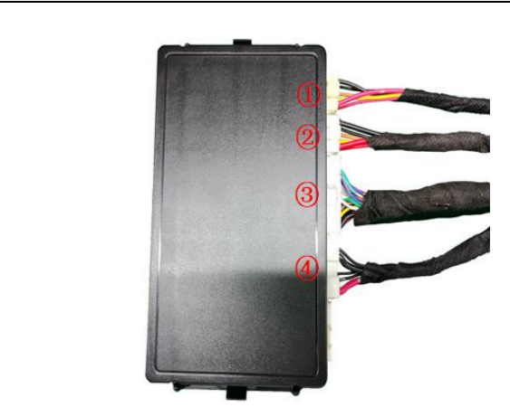
26. Insert the strut wiring harnesses ① ②, lock signal harness ③, and power harness ④ into the ECU in sequence.
