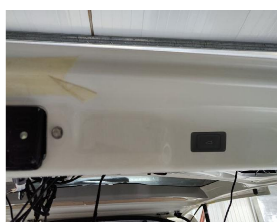
31. Reinstall all the trim panels and install the added tailgate switch.
