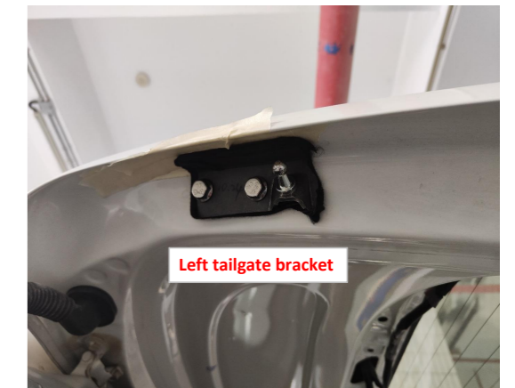
6. Replace the left tailgate bracket.
