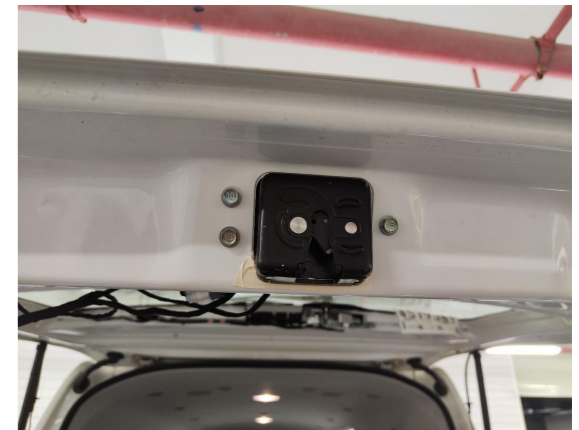
16. Secure the power latch.
