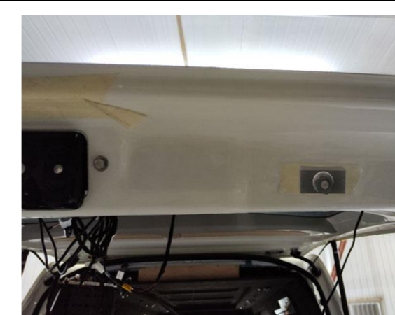
30. Install the hole opener and turn the nut to open the hole.
