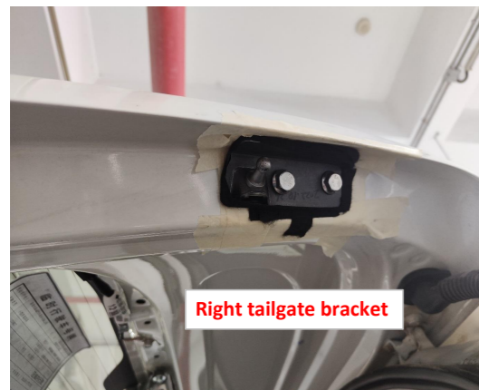
7. Replace the right tailgate bracket.
