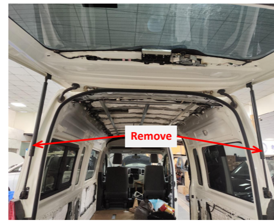
4. Remove the tailgate struts.
