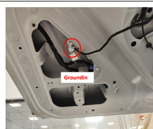
19. Ground at the indicated location on the right side of the tailgate.
