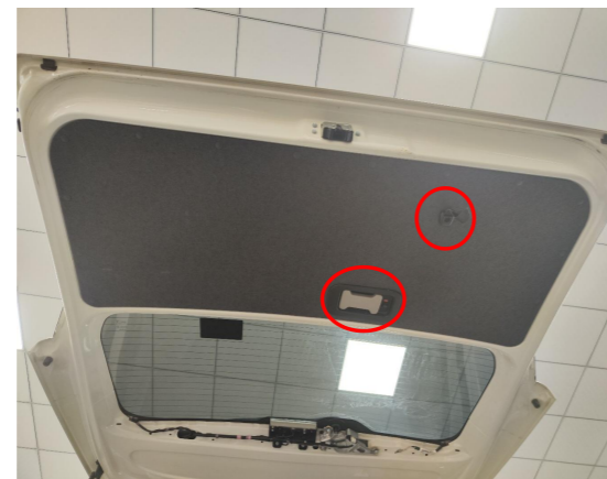
3. Remove the tailgate trim panel.
