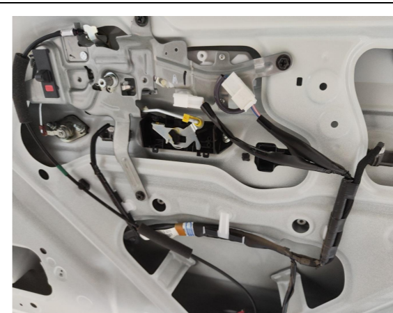
20. Connect the plug of the power harness to the signal plugs at the tailgate.
