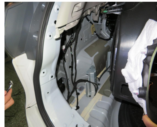
4. Remove the trim panel on the left side of the trunk to allow wiring harnesses to pass through.
