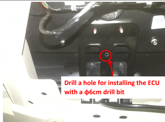
7. Drill a hole at the indicated bracket behind the lock position for installing the ECU (just need to drill through the bracket).
