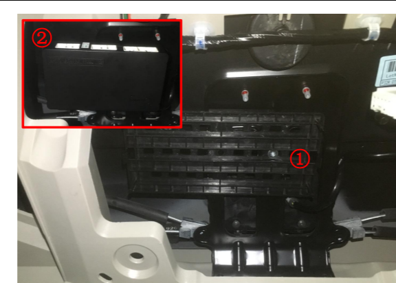
3. Take out the trunk floor mat and remove the screws in the circles from the left side trim panel.
