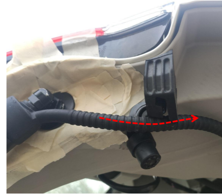
18. Pass the strut wiring harness through the shown position and the drilled hole into the tailgate and then plug the hole with hole plug.
