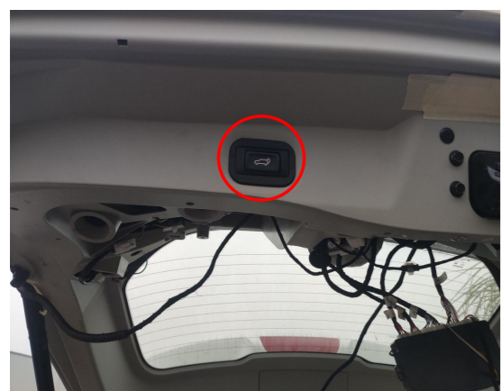
12. Remove the original cover panel and install the added tailgate switch.
