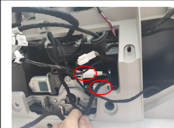
10. Connect the plugs of the lock signal harness to the plugs of the power latch.
