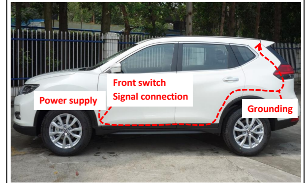
21. Route the power harness as indicated.
