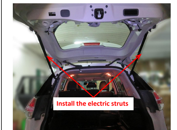
16. Install the electric struts, L on the left, R on the right (the first letter of the strut code).
