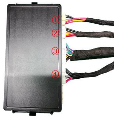
27. Insert the strut wiring harnesses ①②, lock signal harness ③, and power harness ④ into the ECU in sequence and then mount the ECU onto its bracket.
