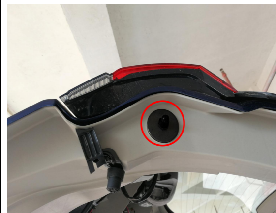
15. Replace the left and right sides ball studs and shims.
