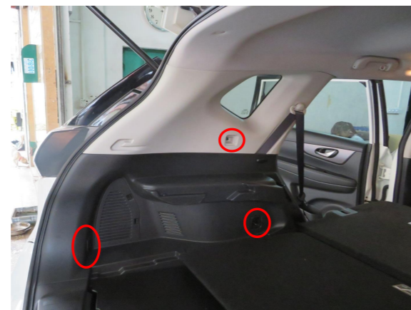
3. Take out the trunk floor mat and remove the screws in the circles from the left side trim panel.
