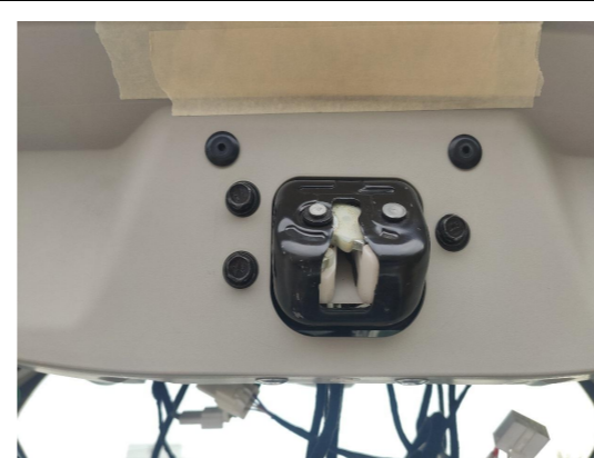
4. Remove the trim panel on the left side of the trunk to allow wiring harnesses to pass through.
