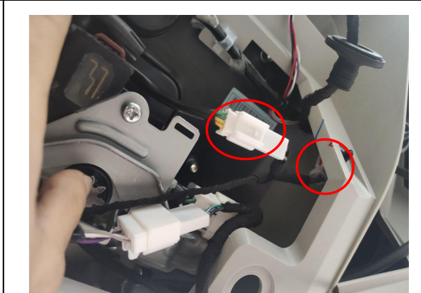
11. Connect the plugs of the lock signal harness to the plugs of the original tailgate switch.
