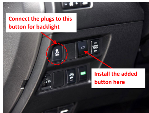
24. Install the added front switch and connect the plugs behind the panel for backlight.
