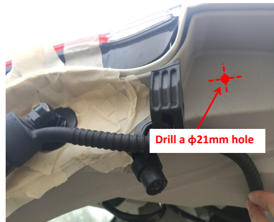
17. Drill a hole at the indicated position using a φ21mm drill bit to allow the strut wiring harness to pass through.
