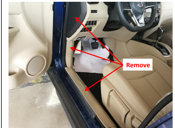
1. Remove the front left triangular trim panel and door sill panels.
