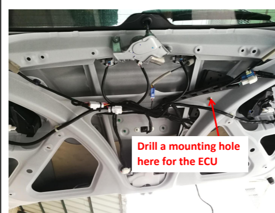
24. Use a φ6mm drill bit to drill a mounting hole at the indicated position for the ECU.
