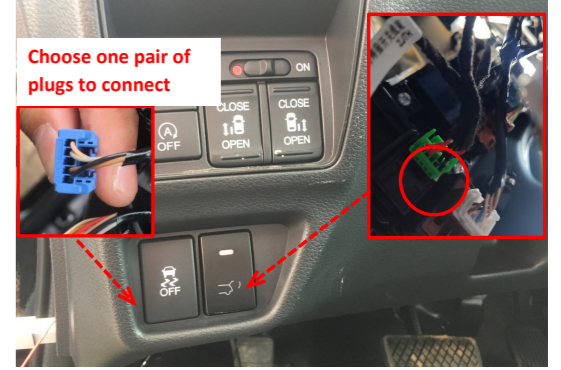
21. Install the added front switch and connect the plugs for backlight (due to configuration differences, two pairs of plugs have been reserved. Choose the correct one pair for connection and pay attention to avoid the plug of multifunction combination button).
