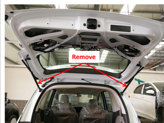
9. Remove the gas struts.
