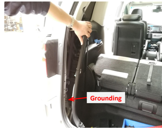
19. Ground at the left side of the trunk.
