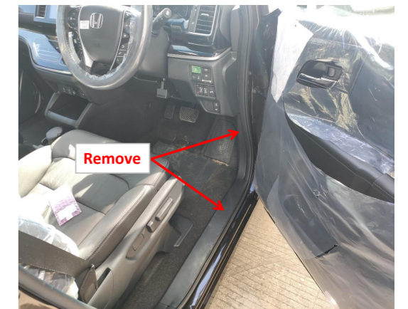
1. Remove the front right side trim panel and door sill panel.
