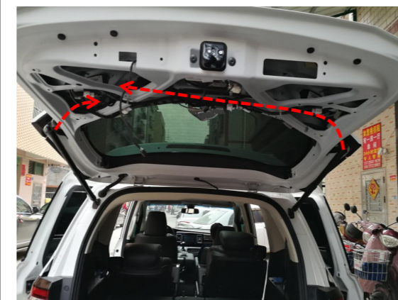
14. Route the strut wiring harnesses.
