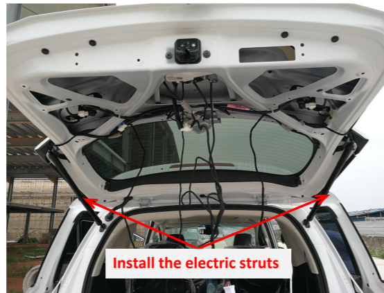
13. Install the electric struts, L on the left and R on the right (the first letter of the strut code).
