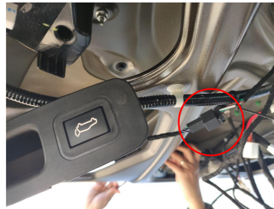
8. Connect the plug of the lock signal harness to the added tailgate switch
