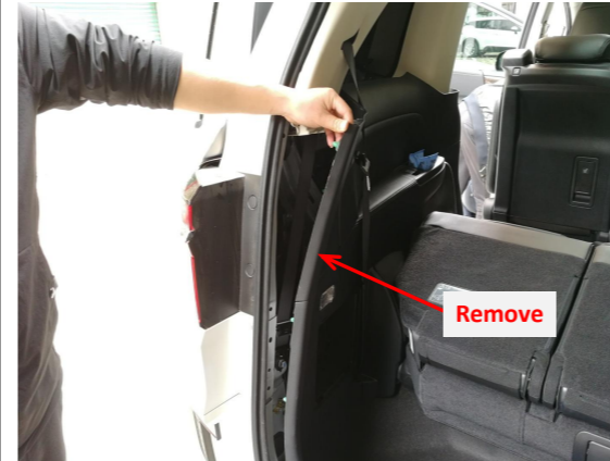
4. Remove the trim panel from the left side of the trunk to allow wiring harnesses to pass through.
