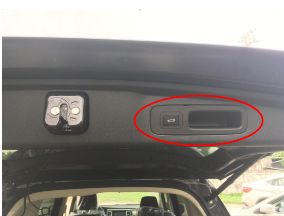
27. Reinstall all the trim panels and install the added tailgate switch.
