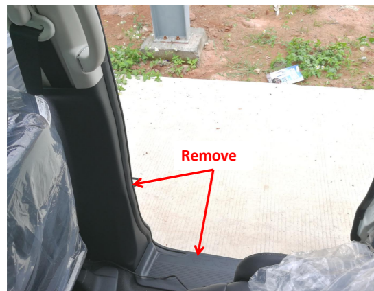
2. Remove the rear right side door sill panel and B-pillar trim panel.
