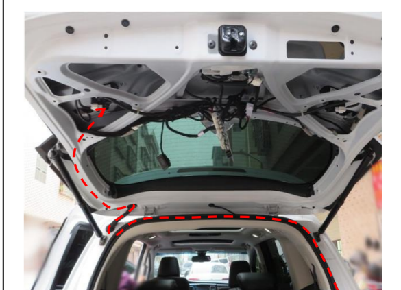
16. Route the power harness to the tailgate.
