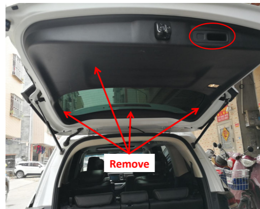
3. Remove the tailgate trim panels.
