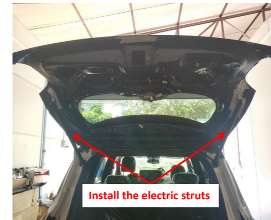
10. Install the electric struts.
