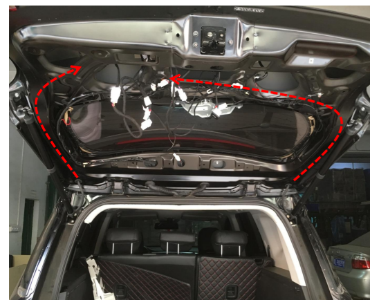
12. Route the left and right strut wiring harness to the tailgate as indicated.
