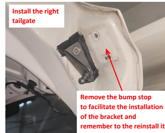
9. Install the right tailgate bracket.
