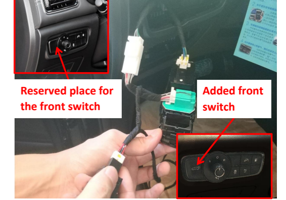
21. (For models that have the reserved place for the front switch) Remove the switch assembly, install the added front switch, connect the plugs and reinstall the switch assembly.
