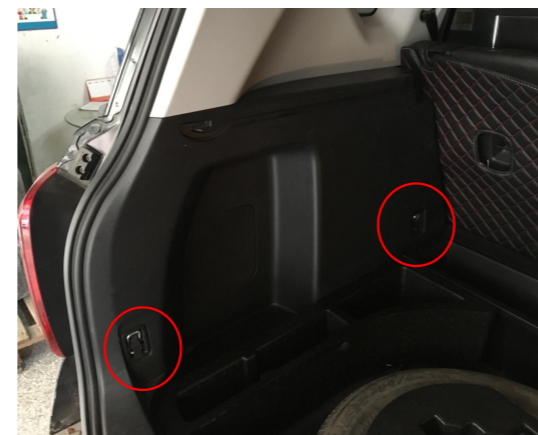
4. Take out the trunk floor mat and remove the indicated trim panel.
