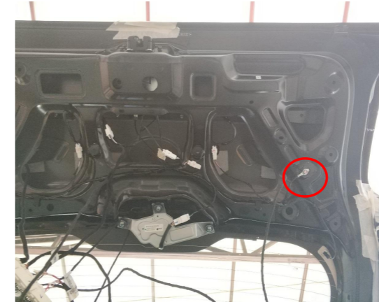
20. Ground at the indicated position on the right side of the tailgate.
