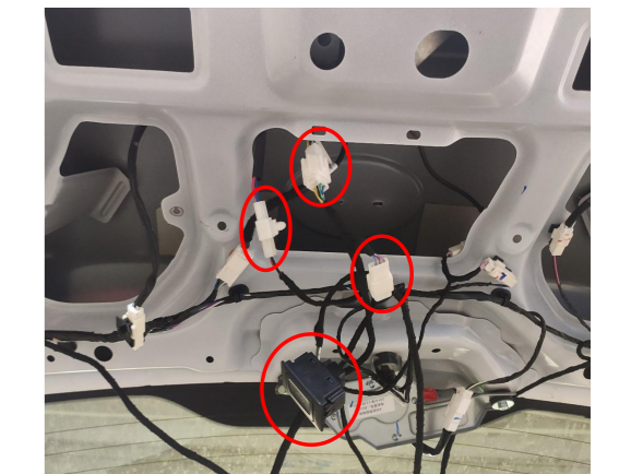
16. Connect the plugs of the lock signal harness to the plugs of the power latch and the added tailgate switch.
