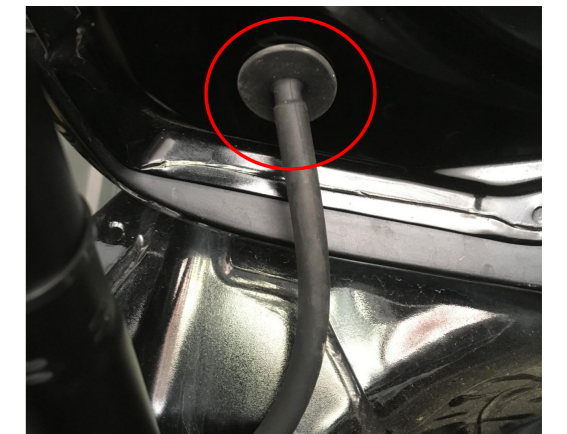
11. Thread the strut wiring harness through the indicated hole, the same on both sides.
