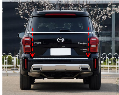
27. Press the added tailgate switch to close the tailgate once, the system completes initialization, and then test each function of the electric tailgate.
