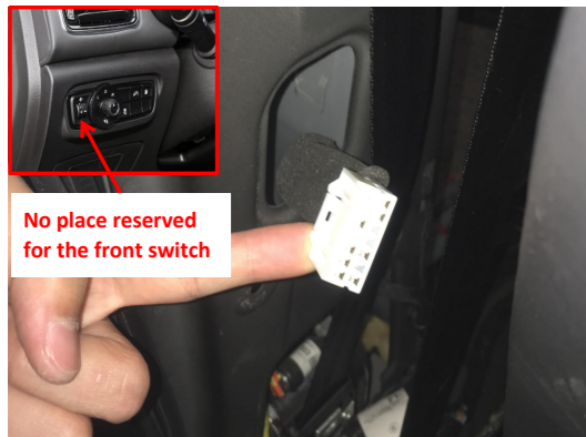
22. (For models that have no reserved place for the front switch, such as GS7) connect the plugs of the power harness to the B-pillar plugs.
