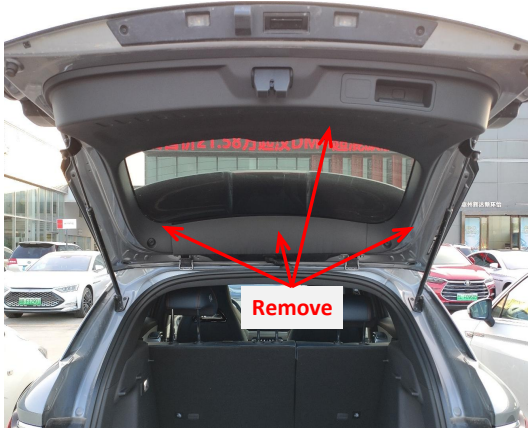
3. Remove the tailgate trim panels.
