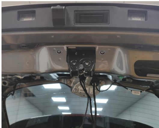
11. Install the power latch and fasten it with provided screws.
