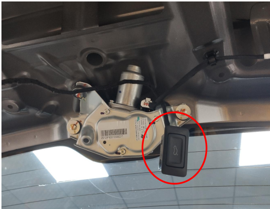
13. Connect to the added tailgate switch.
