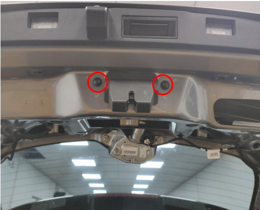
9. Remove the original latch.
