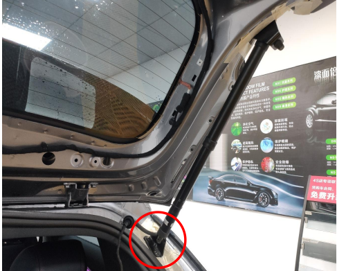
6. Install the electric struts, L on the left and R on the right (the first letter of the strut code), making sure the ends with wiring harnesses are on the vehicle body.
