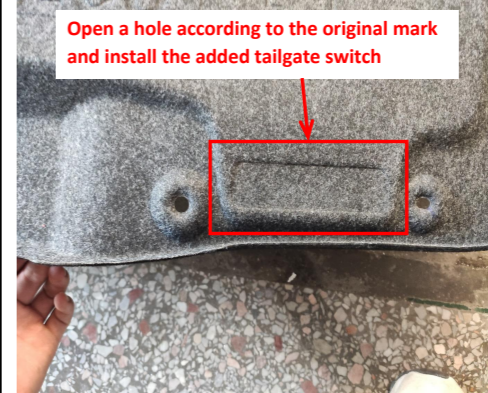
37. Install the added switch at the reserved place.
