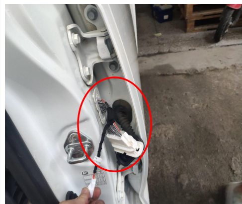
27. Connect the plugs of the power harness to the B-pillar signal plugs at the rear left B-pillar.
