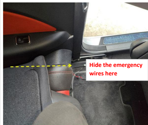
22. Wrap the two emergency wires of lock and hide them under the left side of the rear seat.
