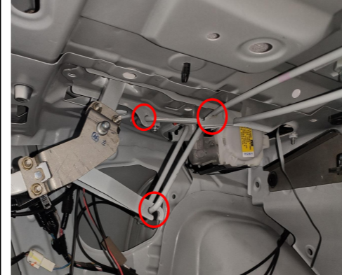
36. Apply a little grease to the place where the torsion spring contacts with the body sheet metal to prevent noise during operation.
