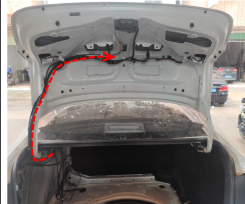
24. Route the power harness from the driver's area to the trunk and then route to the tailgate along the hinge.
