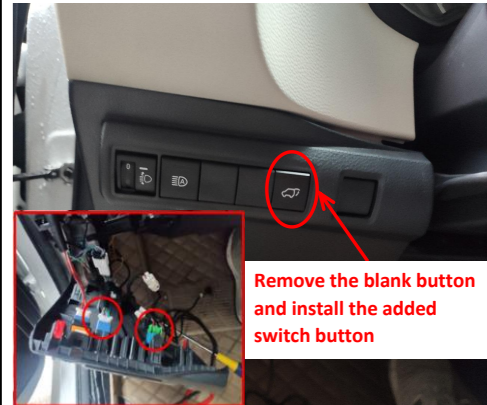
26. Remove the blank button and install the added switch button. Connect the plug to the button beside for backlight.
