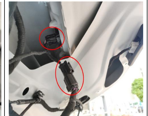
20. Connect the plugs of the lock signal harness to the original tailgate switch.
