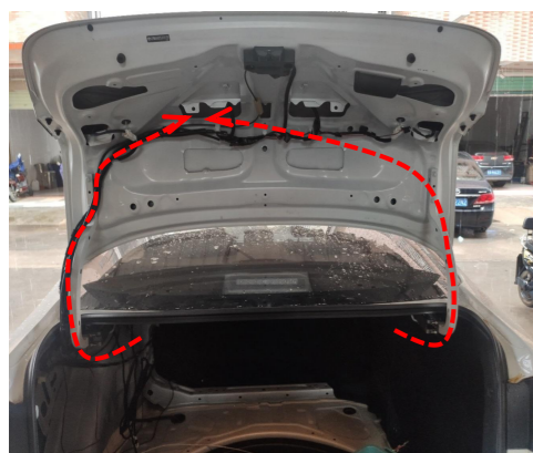
15. Route the strut wiring harnesses to the tailgate along the hinges.
