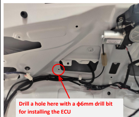
31. Drill a hole at the indicated location with a \phi 6\text{mm} drill bit for installing the ECU.
