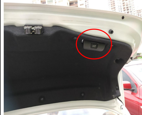
38. Reinstall all trim panels and install the added tailgate switch.
