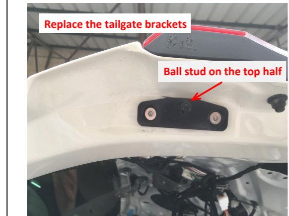
8. Replace the left and right tailgate brackets with the ball studs on the top half.
