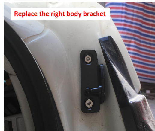
7. Replace the right body bracket.
