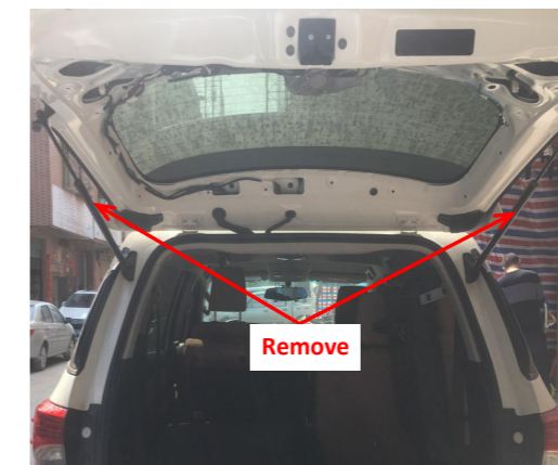
5. Remove the original gas struts.
