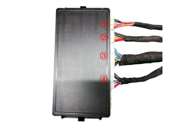
26. Insert the strut wiring harnesses ①②, lock signal harness ③, and power harness ④ into the ECU in sequence, and mount the ECU on its bracket.
