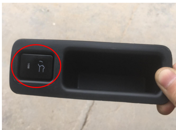
28. Install the added tailgate switch button on the tailgate handle.
