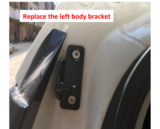
6. Replace the left body bracket.
