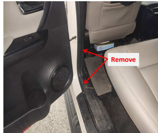
2. Remove the rear left side door sill panel and B-pillar trim panel.
