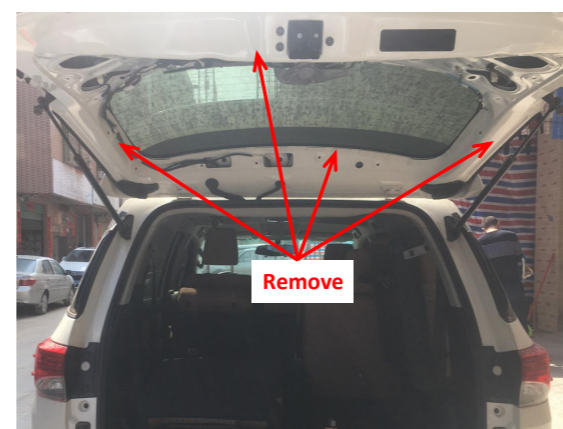
4. Remove the tailgate trim panels.
