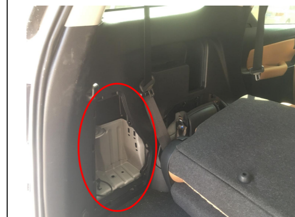
3. Remove the trim panel on the left side of the trunk to allow wiring harnesses to pass through.
