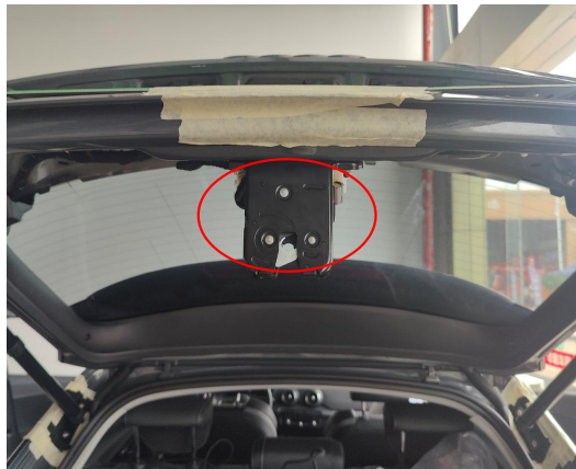
9. Remove the original latch and install our power latch.
