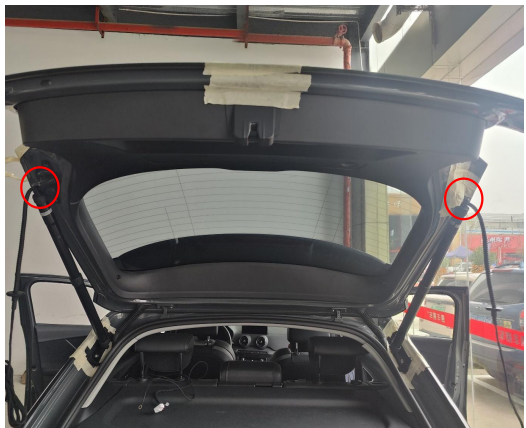
15. Install the electric struts, L on the left R on the right (the first letter of the strut code).
