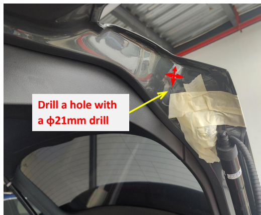
16. Drill a hole at the indicated position on both sides of the tailgate with a φ21mm drill bit.
