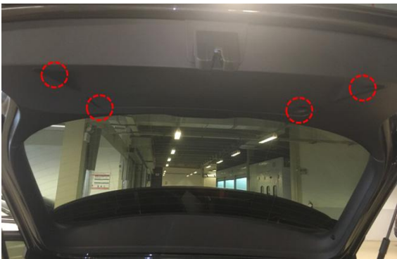
3. Remove the screws on the tailgate trim panel.
