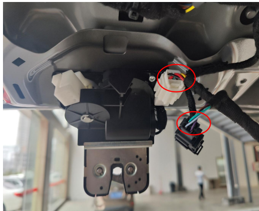
11. Connect the plugs of the lock signal harness to the power latch.
