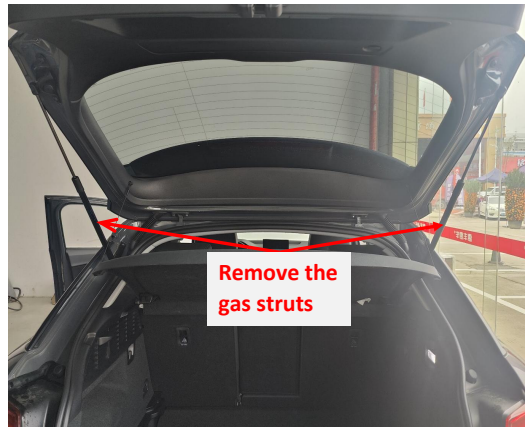
13. Remove the gas struts.
