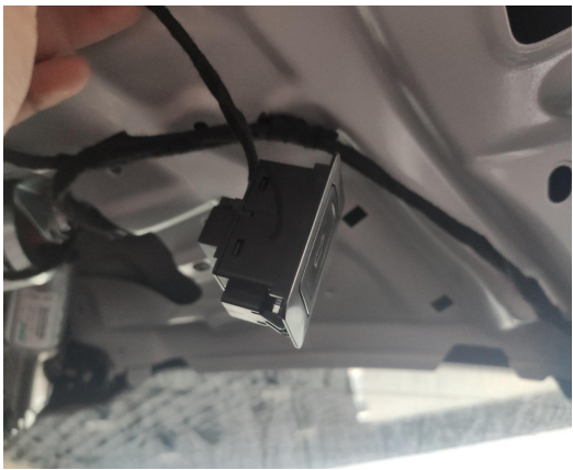
12. Connect the plug of lock signal harness to the added tailgate switch.
