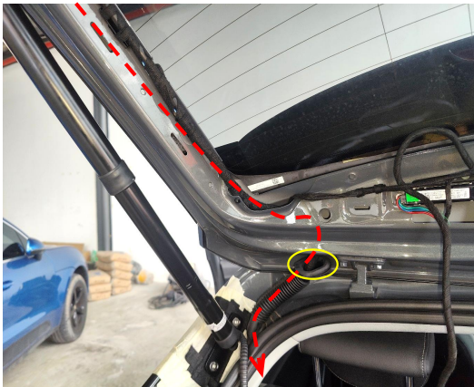
7. Thread the lock signal harness to the left side of the trunk through the original rubber tube.(no plug connection for now)
