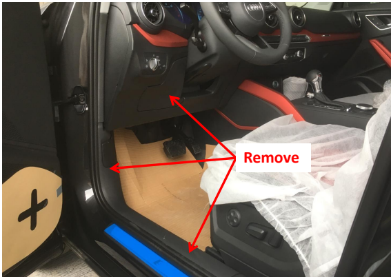
1. Remove the front left side trim panel, door sill panel and storage box.
