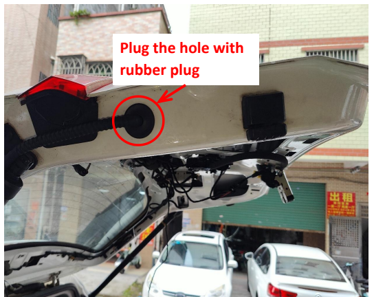
13. Plug the holes on both sides with the rubber plugs.
