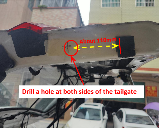
10. Mark the positions to be drilled with tape and pay attention to avoid the taillights.
