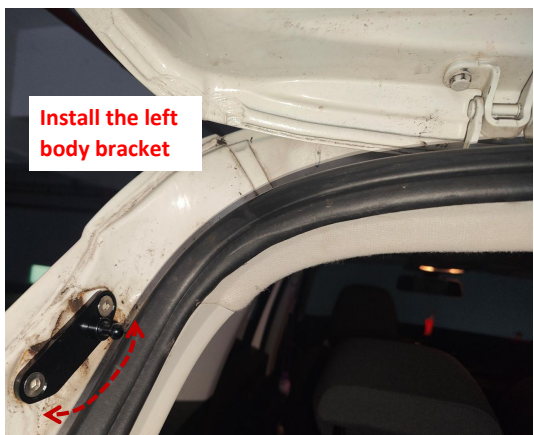
5. Install the left body bracke with the curved edge facing down.
