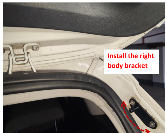
6. Install the right body bracke with the curved edge facing down.
