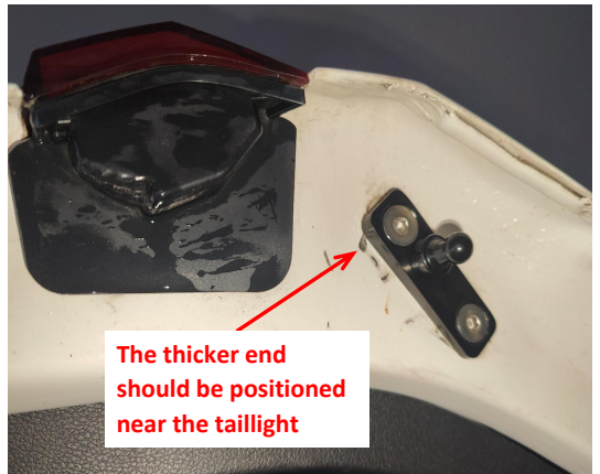
8. Install the right tailgate bracket. The thicker end of the bracket should be positioned near the taillight.
