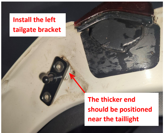
7. Install the left tailgate bracket. The thicker end of the bracket should be positioned near the taillight.
