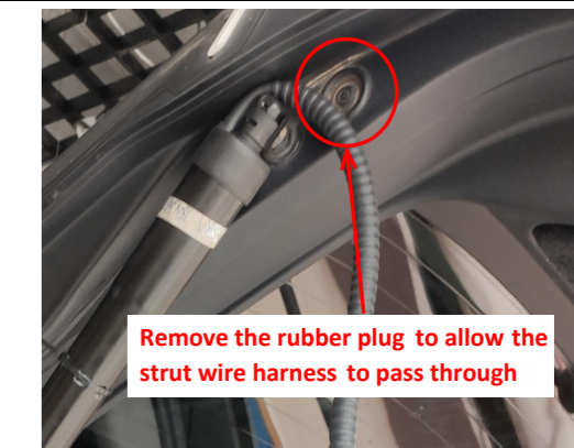
6. Remove the indicated rubber plug to allow the strut wiring harness to pass through and then plug hole tightly. Both sides follow the same method.
