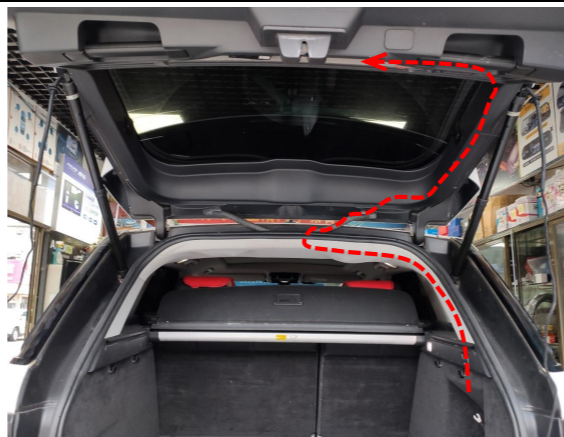
14. Route the power harness to the tailgate (wiring only, no power or plug connection).
