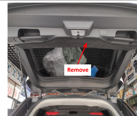
1. Remove the tailgate trim panels.
