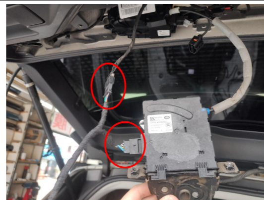
9. Remove the original power latch(for easy connection of the plugs), connect the plugs of the lock signal harness to the power latch and then put the power latch back.
