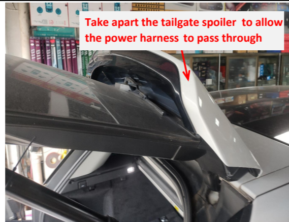
13. Disassemble the spoiler to allow the power harness to pass through.
