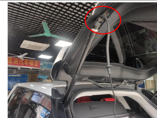
5. Install the electric struts, L on the left and R on the right (the first letter of the strut code), making sure the ends with wiring harnesses are on the tailgate.
