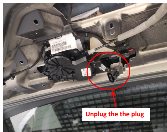
8. Unplug the indicated plug from the original power latch.
