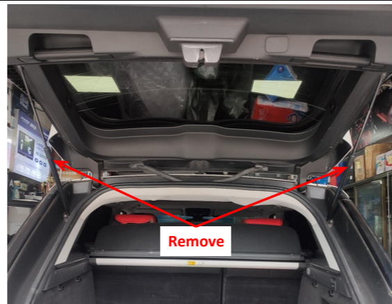
4. Remove the original gas struts.
