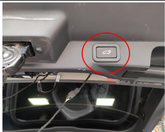
12. Install the added tailgate switch (remove the original cover panel here).
