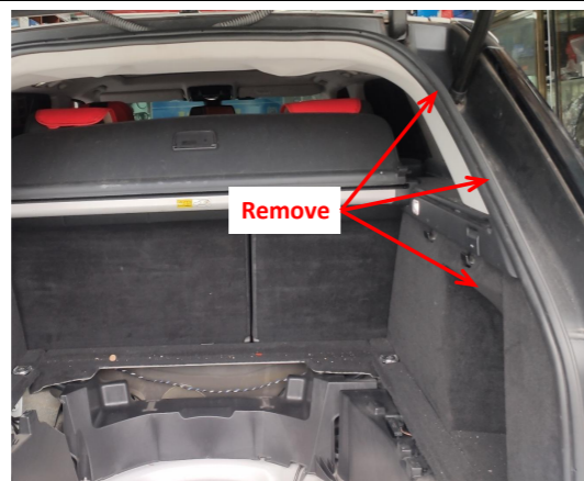
3. Remove the trim panel from the right side of the trunk to allow the power harness to pass through.
