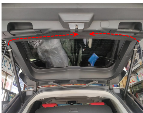
7. Route the strut wiring harnesses to the tailgate.
