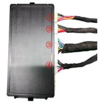
31. Insert the left and right strut wire harnesses  $\widehat{\mathbb{1}}\widehat{\mathbb{2}}$  , lock signal harness (3), and power harness (4) into the ECU in sequence.
