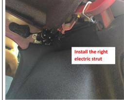
19. Install the right electric strut (the first letter of the strut number shows the left and right) .
