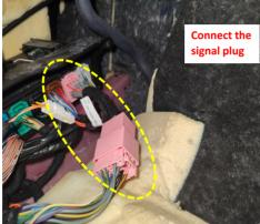
28. Remove the original pink plug and plug our signal plug into its socket.
