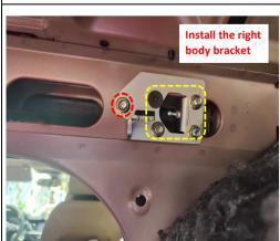
15. Use a bolt and nut (as indicated by the red circle) to secure the bracket first.
