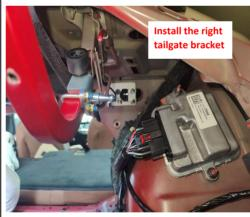
12. Install the right tailgate bracket. Install the provided bump stop to secure the bracket and then install the U-
