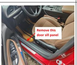
3. Remove the front left door sill panel and lift up the floor mat to find out the fuse box.
