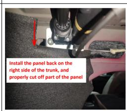
34. Install the panel back on the right side of the trunk, and properly cut off part of the panel that interfere with the operation of the strut.
