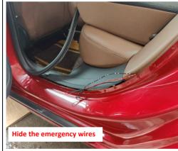
10. Route the emergency wires from the trunk to the left side of rear seats and hide them under the door sill nanel
