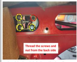
18. Thread the three bolts(indicated by the yellow circles) through the bracket from the back side, use nuts to secure them and use another nut to secure the countersunk screw.
