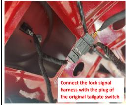
9. Connect the lock signal harness with the plug of the original tailgate switch.
