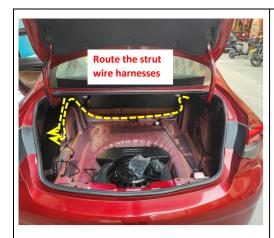
21. Route the left and right strut wire harnesses to the left side of the trunk along with the original wires.
