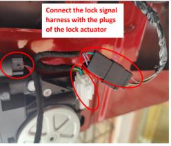
7. Connect the lock signal harness with the plugs of the lock actuator.
