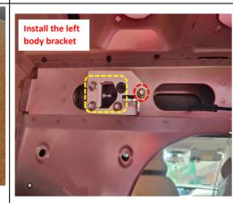
17. Use a bolt and nut (as indicated by the red circle) to secure the bracket first.
