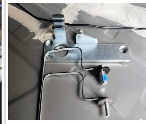
6. Fold the handle of the screw into the shape as shown above for easy insertion into the holes.
