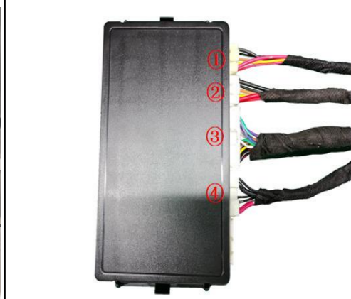
32. Insert the strut wiring harnesses ①②, lock signal harness ③, and power harness ④ into the ECU in sequence.
