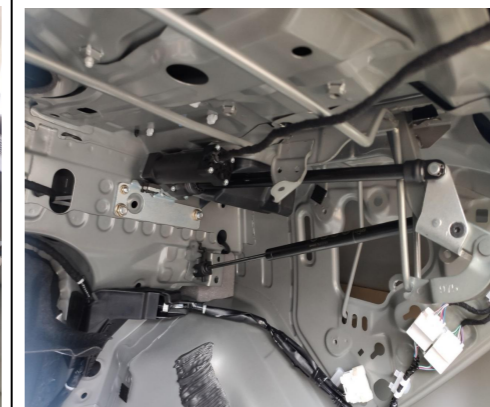
13. Install the electric struts, L on the left and R on the right (the first letter of the strut code), making sure the ends with wiring harnesses are on the car body.
