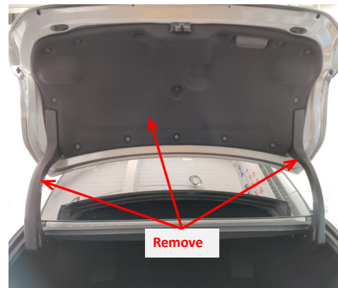
3. Remove the tailgate trim panels.
