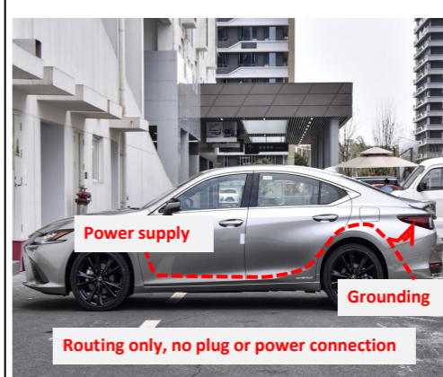
25. Route the power harness as indicated.
