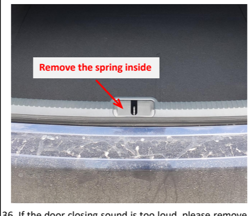
36. If the door closing sound is too loud, please remove the spring from the dust seal at the striker to prevent it from touching the electric lock by making the dust seal lose its elasticity.
