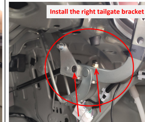
12. Install the right tailgate bracket at the right hinge.
