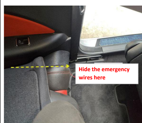
24. Wrap the two emergency wires with electric tape and hide them under the rear left side trim panel.
