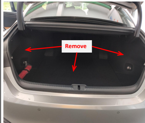
4. Remove the trunk liner and adjust the position of the spring on the left side of the trunk.
