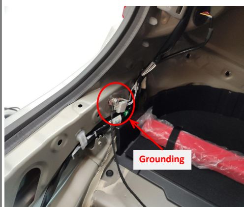
27. Ground at the left side of the trunk.
