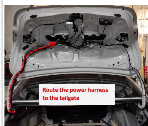
26. Route the power harness to the tailgate.
