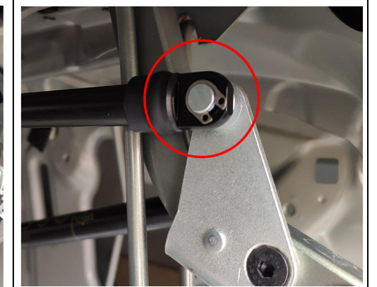
14. Use the circle clip to secure the strut; the same on both struts.
