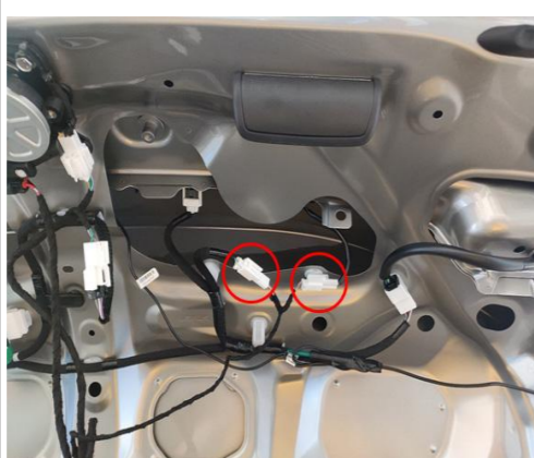
22. Connect the lock signal harness to the plugs of the original tailgate switch.
