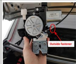
19. Mount the emergency cable onto the indicated fastener of our power latch (remove the fastener of the emergency cable from the tailgate first).
