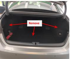
4. Remove the trunk liner and adjust the position of the spring on the left side of the trunk.
