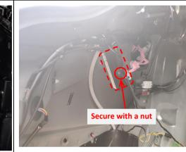
32. Remove the wire clip from the indicated hole, install the ECU at the hole and secure it with a nut.
