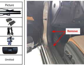
. Remove the front left side trim panel and door sill panel.
