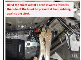
15. Bend the sheet metal a little inwards towards the side of the trunk to prevent it from rubbing against the strut. Both the left and right sides are the same.
