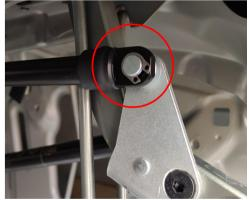
14. Use the circle clip to secure the strut; the same on both struts.
