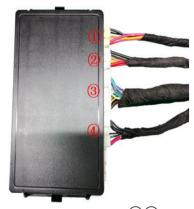
33. Insert the strut wiring harnesses (1)(2), lock signal harness (3), and power harness (4) into the 34. Check whether the power latch and the ECU in sequence.
