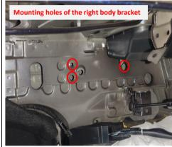
8. Locate the mounting holes of the right body bracket.
