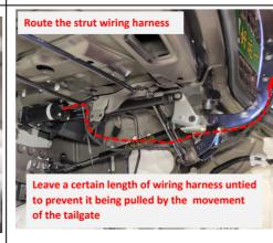
17. Route the strut wiring harnesses along the hinges to the tailgate and tie them along with the original wiring harnesses.
