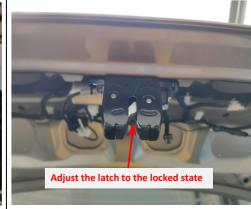
20. Install the power latch and adjust the latch to the locked state by hand to prevent accidental closing during the installation process.
