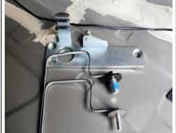
6. Fold the handle of the screw into the shape as shown above for easy insertion into the holes.
