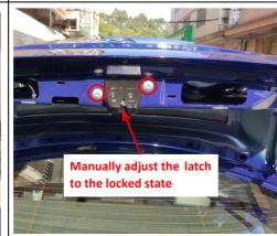
17. Remove the original latch, install our power latch, and then manually adjust the latch to the locked state.
