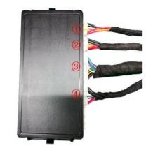
28. Insert the strut wiring harnesses (1)(2), lock signal harness ③, and power harness ④ into the open the tailgate. The system will complete initialization, ECU in sequence.
