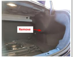
7. Remove the trunk liner and the trim panels on both sides of the trunk.
