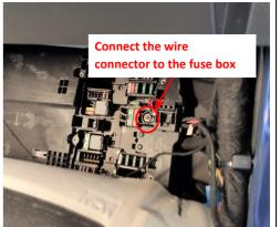
25. Connect the wire connector to the fuse box (fasten with a nut) for power supply and then put 26. Remove the indicated cable clip for securing the fuse box cover back.
