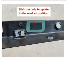
33. Stick to hole template to the marked position. 34. Open the hole.
