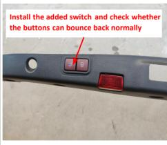
35. Install the added tailgate switch and check whether the buttons can bounce back normally.
