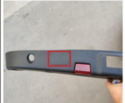
30. Open a hole at the indicated position for installing the added tailgate switch.
