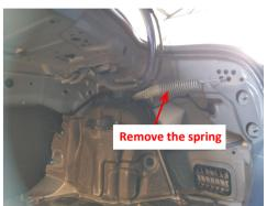
8. Remove the left and right springs from the trunk.
