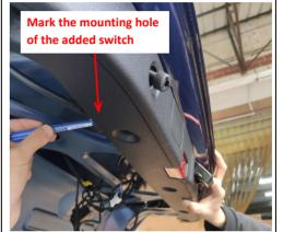
31 Fasten the trim panel to the tailgate and align the hole to be opened with the sheet metal hole.
