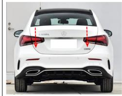
29. Manually close the tailgate until the latch touches the striker, then press the original tailgate switch to and then test each function of the electric tailgate.
