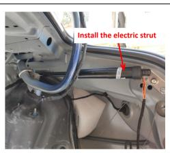
14. Install the electric struts, L on the left and R on the right (the first letter of the strut code), making sure the ends with wiring harnesses point outward.
