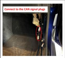
24. Connect the plugs of power harness to the CAN signal plugs.
