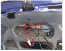
18. Connect the plugs of lock signal harness to the plugs of original tailgate switch and the added plugs of the power latch.
