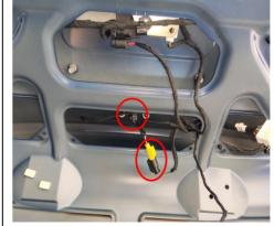
19. Connect the plugs of lock signal harness to the switch.
