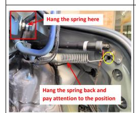
15. Hang the springs back with the long ends hanging on the car body.
