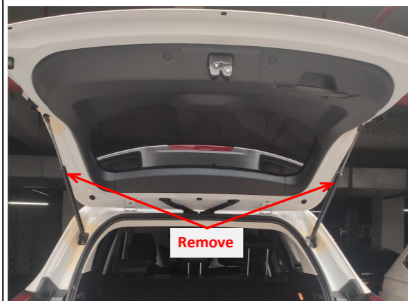
8. Remove the original gas struts.
