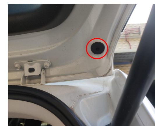
13. Thread the strut wiring harness through the indicated hole into the tailgate; both sides are the same.
