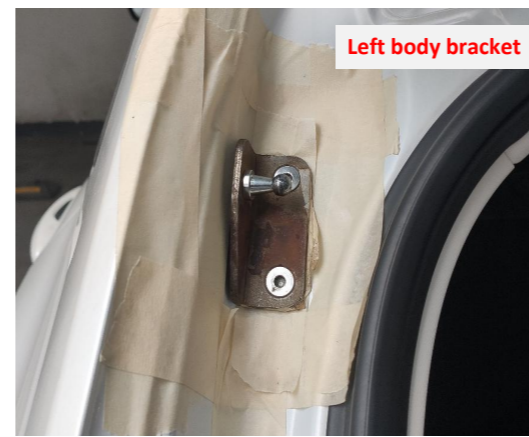
9. Replace the left body bracket.
