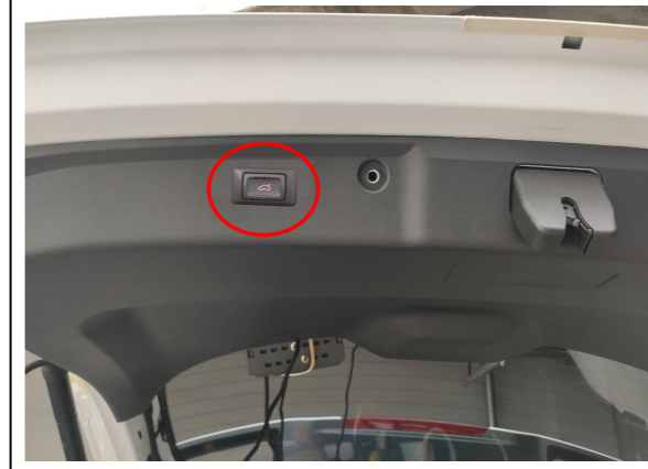
30. Install the added tailgate switch and reinstall all trim panels.
