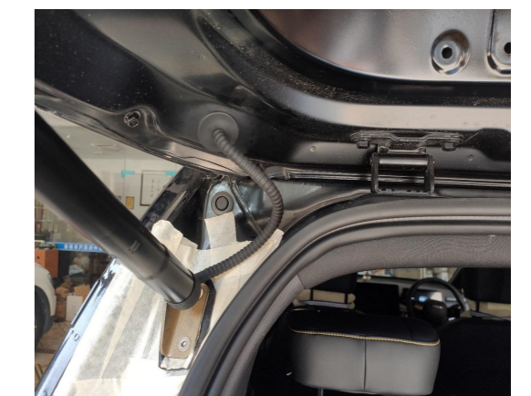
16. Plug the hole securely.
