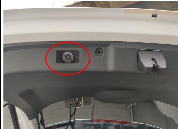
28. Install the hole opener.
