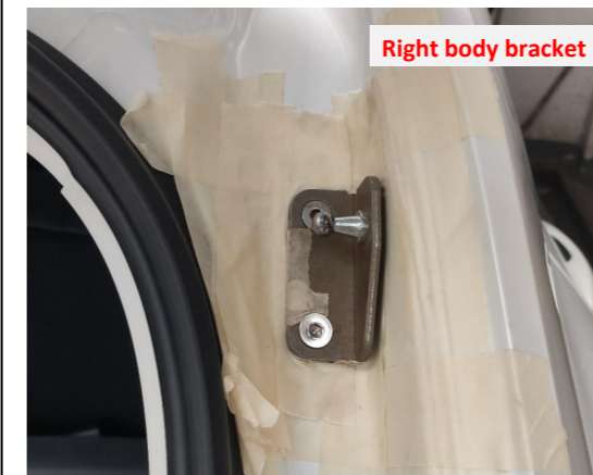
10. Replace the right body bracket.
