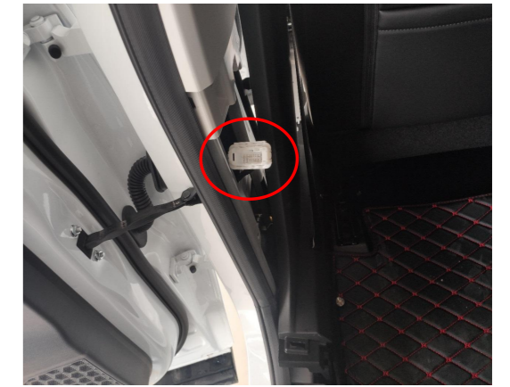
21. Connect the power harness to the B-pillar plugs at the rear left side B-pillar.
