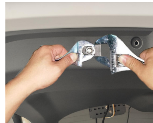
29. Open the hole (one hand holds the wrench, the other turns the nut).
