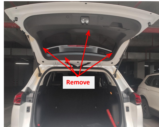
3. Remove the tailgate trim panels.
