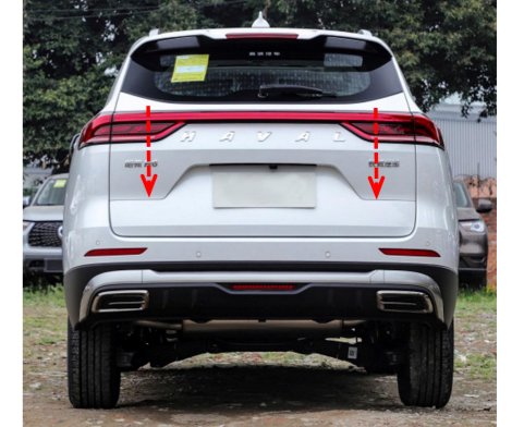
26. Press the added tailgate switch button to open and close the tailgate once for initializing the system, and then test each function of the electric tailgate.
