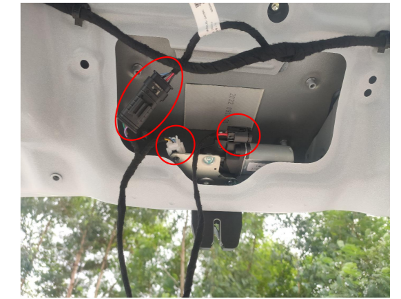
6. Connect the lock signal harness to the plugs of the power latch.
