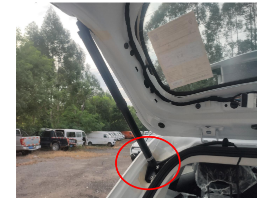
12. Install the electric struts, L on the left and R on the right (the first letter of the strut code), making sure the ends with wiring harnesses are on the vehicle body.
