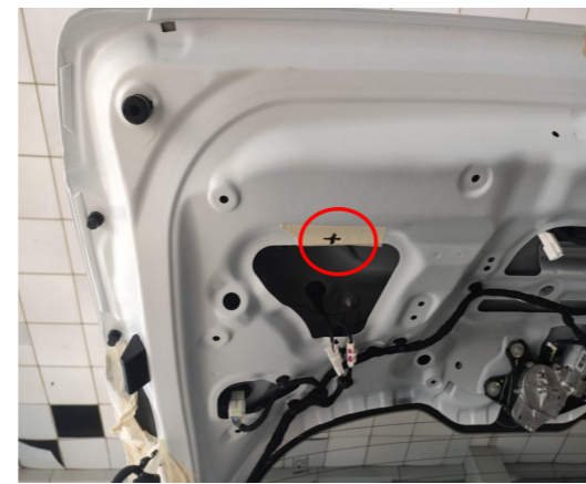
24. Drill a hole at the indicated position with a \phi 6 mm drill bit and fix the ECU to the hole.
