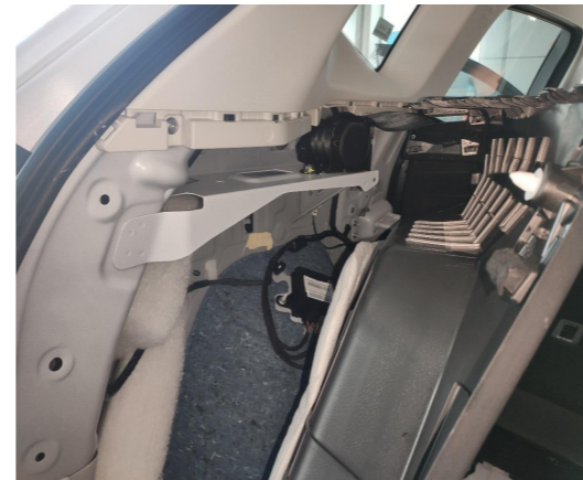
4. Remove the trunk floor mat and storage box. Separate the trim panel on the left side to allow wiring harnesses to pass through.
