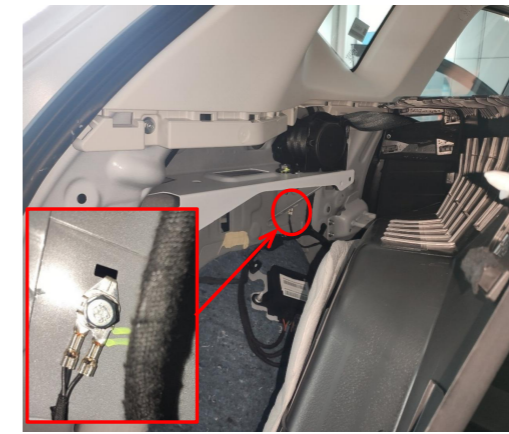
20. Ground at the left side of the trunk.
