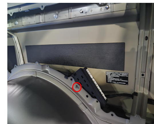
25. Secure the ECU at the indicated position.
