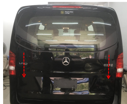
27. Press the added tailgate switch to close the tailgate once, and then test each function of the electric tailgate.
