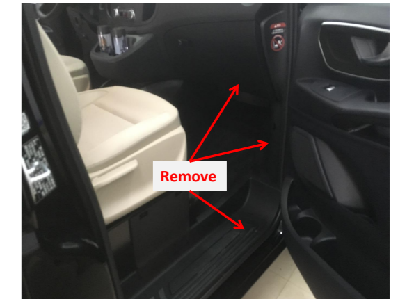
1. Remove the indicated front right side trim panels and step board.
