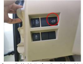
25. Remove the blank button from the switch panel, install the added front switch and connect to the plugs of the switch beside it for backlight.
