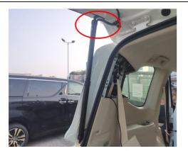
13. Install the electric struts, L on the left and R on the right the first letter of the strut code), making sure the ends with 14. Pass the strut wiring harnesses through the original car wiring harnesses are on the tailgate.
