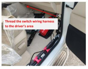
24. Thread the switch wiring harness to the driver's area.
