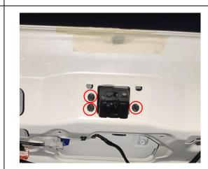
16. Remove the original latch and install the power latch.
