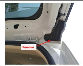
5. Remove the indicated rubber pad to allow the strut wiring harness to pass through. Both sides are the same.
