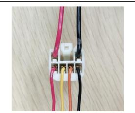
15. Insert the strut wiring harness terminals into the wiring harness connector as shown above.
