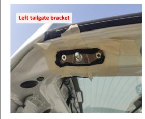
11. Install the bracket on the left side of the tailgate.
