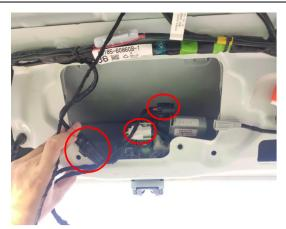
17. Connect the plugs of lock signal harness to the power latch.
