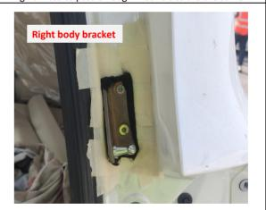
10. Install the bracket on the right side of the vehicle body.
