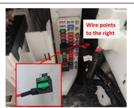
27. Move the original fuse from the fuse box to the fuse tap and plug the fuse tap into the fuse box with wire pointing to 28. Place the ECU at the indicated position and secure it the right.
