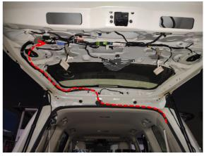
20. Thread the power harness to the tailgate (do not connect ugs before inserting terminals into wiring harness connector).
