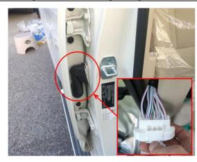
23. Connect B-pillar signal at the rear right side B-pillar.
