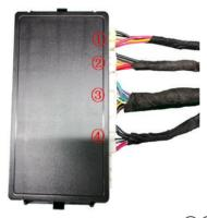
29. Insert the left and right strut wiring harnesses (1)(2), lock signal harness 3, and power harness 4 into the ECU in sequence.
