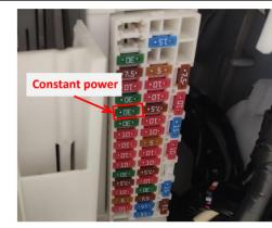
26. The fuse box is on the right side of the front passenger seat and the fuse slot for power supply is indicated above.
