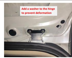
6. Add a washer to the hinges on both sides of the tailgate and secure them with provided screws.
