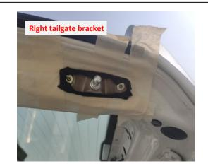
12. Install the bracket on the right side of the tailgate.
