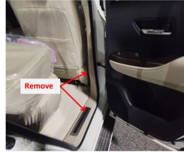
2. Remove the rear right B-pillar trim panel and door sill
