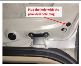
7. Plug the holes on both sides with the provided hole plugs. 8. Remove the original gas struts.
