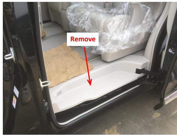
2. Remove the rear left footstep.
