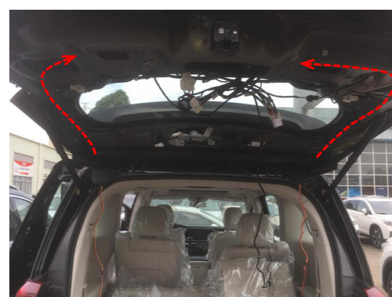
14. Route the strut wiring harnesses as indicated.
