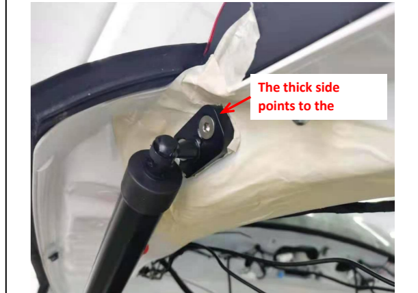
11. Replace the tailgate brackets.
