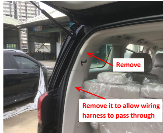
3. Remove the indicated trim panels on the left side of the trunk.
