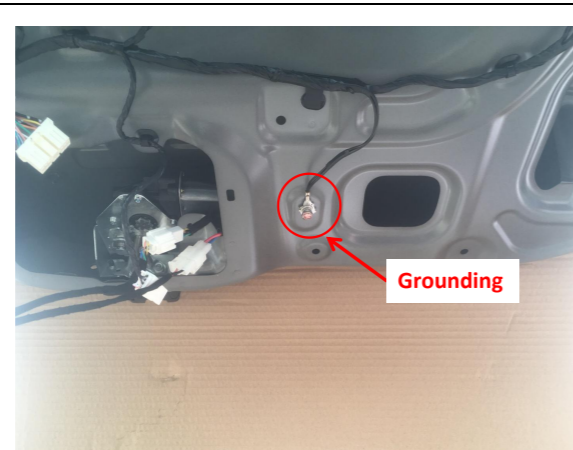
18. Ground at the indicated position.
