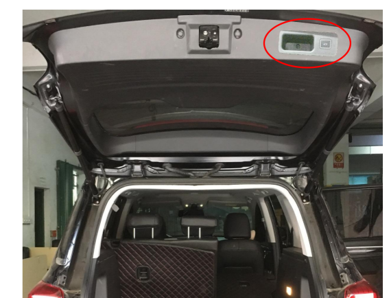
26. Install the added tailgate switch and reinstall all the trim panels.
