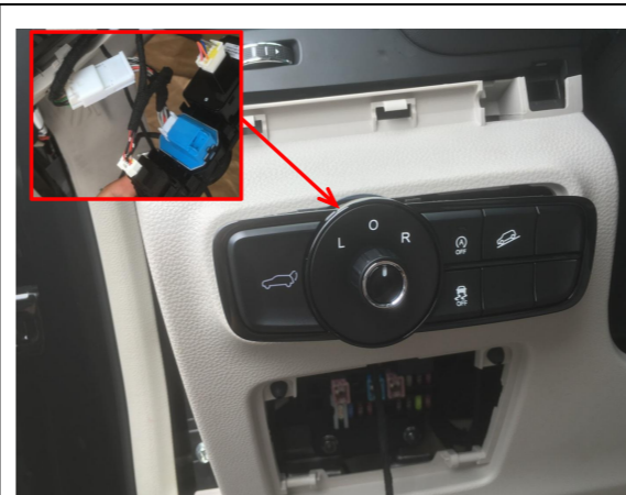
19. Install the front switch as indicated in the diagram.
