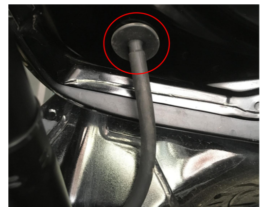
13. Thread the strut wiring harness through the indicated hole into the tailgate.
