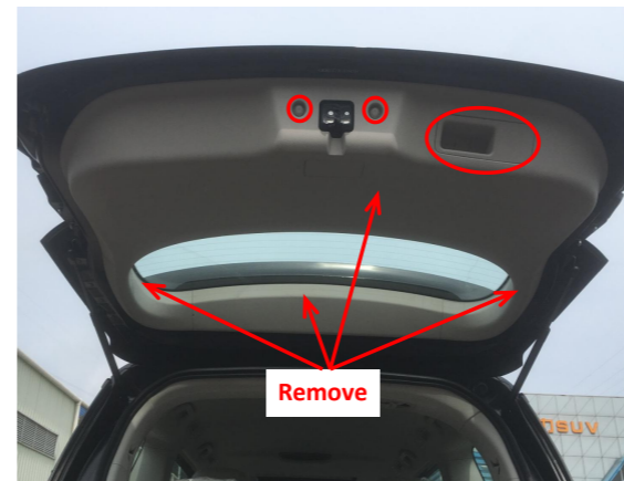
4. Remove the tailgate trim panels.
