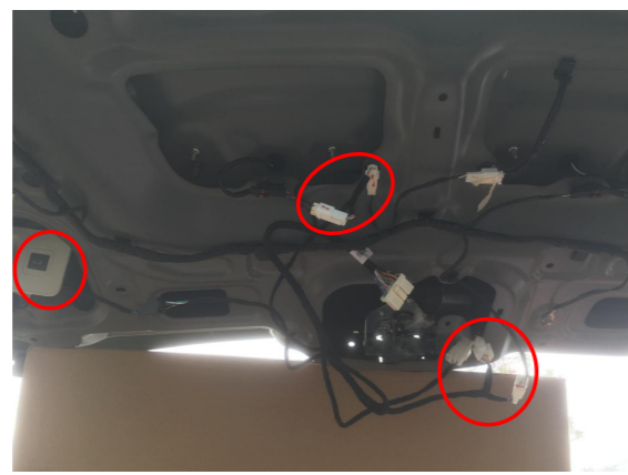
8. Connect the plugs of the lock signal harness to the plugs of the power latch and the added tailgate switch.
