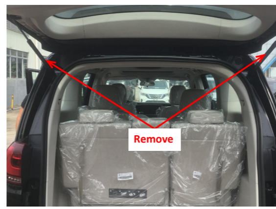
9. Remove the original gas struts.
