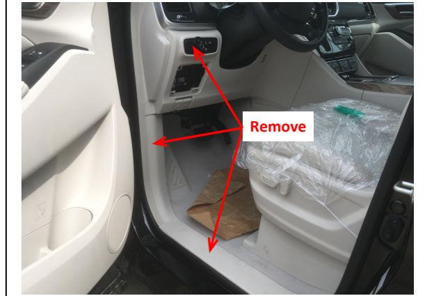
1. Remove the indicated driver's side trim panels.
