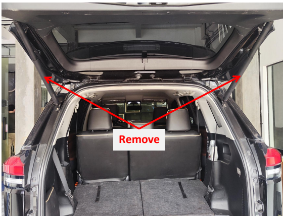
5. Remove the original struts.
