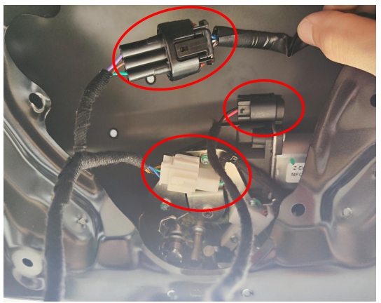
13. Connect the T-harness connectors of the lock signal harness to the connectors of the power latch.
