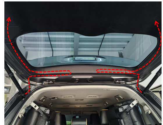
10. Thread the strut wire harnesses through the holes into the tailgate and route them as indicated.
