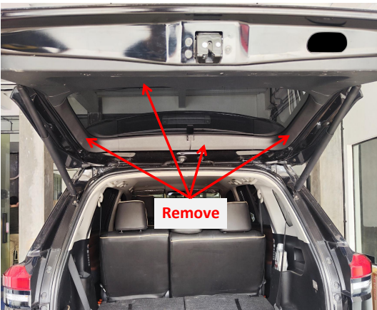
4. Remove the tailgate trim panels.
