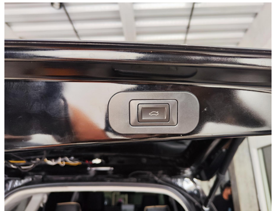
15. Install the added tailgate switch.
