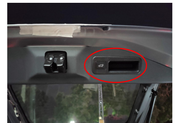
28. Reinstall all trim panels and install the added tailgate switch (remove the original handle).
