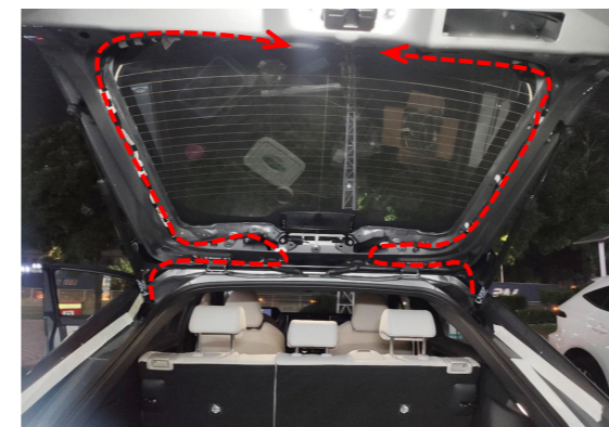
9. Thread the strut wiring harnesses through the original holes into the tailgate and route the wiring harnesses as shown above.
