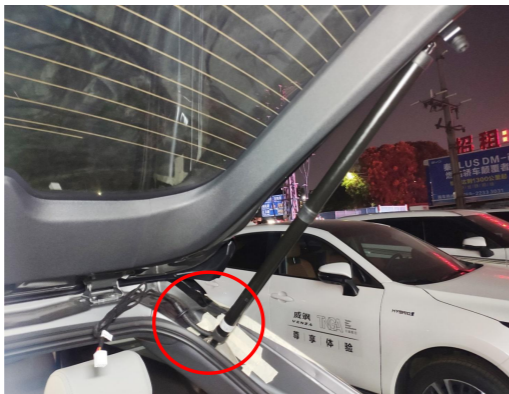
8. Install the electric struts, L on the left and R on the right (the first letter of the strut code), making sure the ends with wiring harnesses are on the car body.
