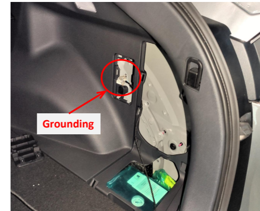
20. Ground at the right side of the trunk.
