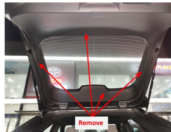
4. Remove the tailgate trim panels.
