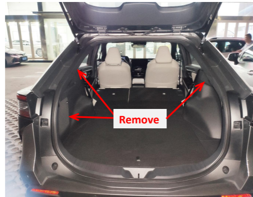
3. Take out the trunk floor mat and foam storage box. Remove the trim panels on both sides of the trunk to allow wiring harnesses to pass through.
