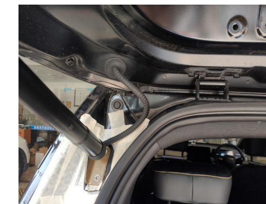
12. Leave a certain length of the rubber tube outside to prevent it from being bent during the movement of the tailgate.
