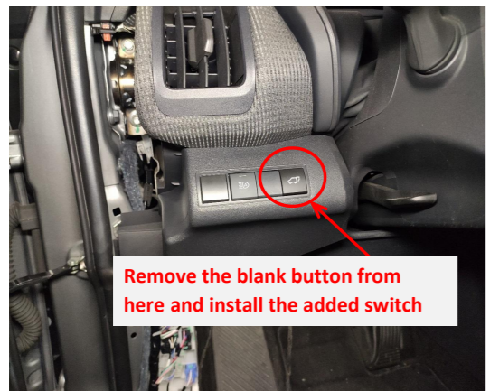
22. Remove the blank button, install the added front switch and connect to the plugs beside the switch for backlight.
