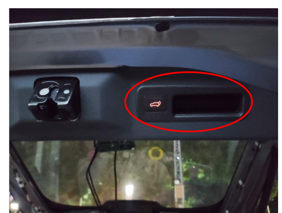
16. Connect the plug of the lock signal harness to the added tailgate switch.
