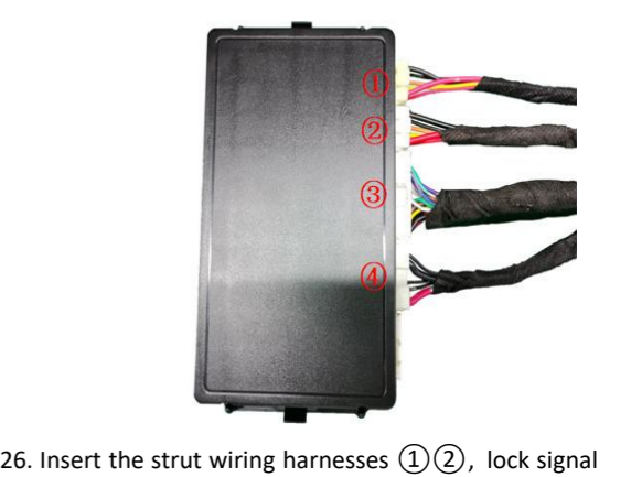
26. Insert the strut wiring harnesses ①②, lock signal harness ③, and power harness ④ into the ECU in sequence, and mount the ECU onto its bracket.
