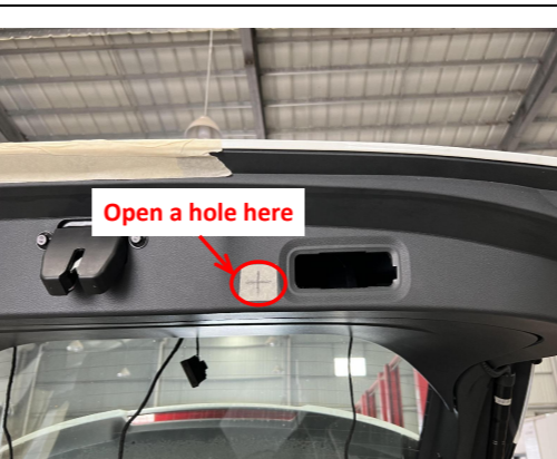
29. Open a hole at the indicated position with a \phi 21\text{mm} drill bit for the added tailgate switch.
