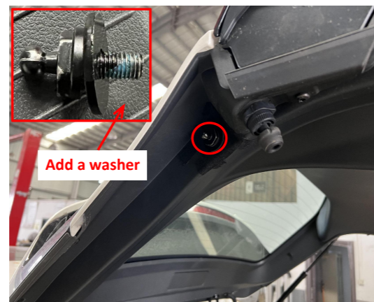
8. Replace the ball studs on both sides of tailgate and add a washer under them.
