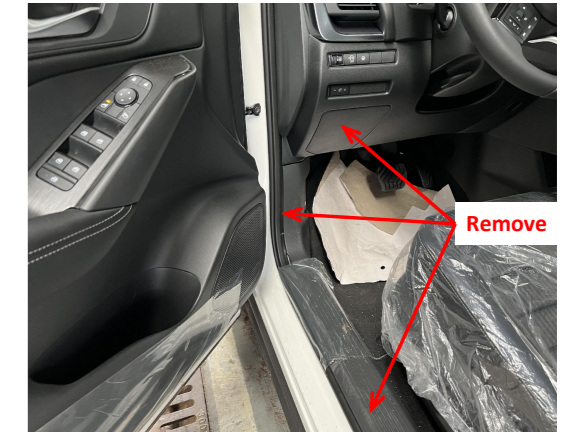
1. Remove the front left door sill panel and the trim panel of fuse box.
