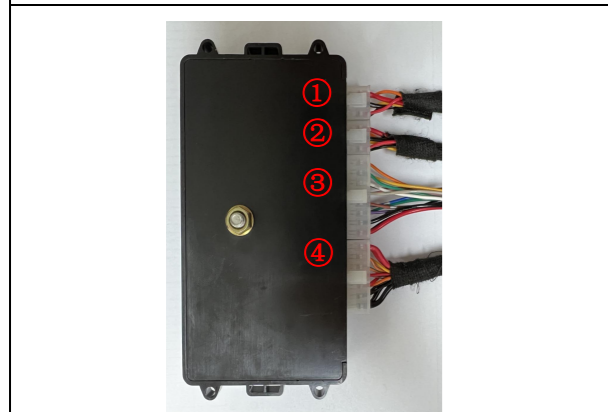
27. Insert the left and right strut wiring harnesses ①②, lock signal harness ③, and power harness ④ into the ECU in sequence.
