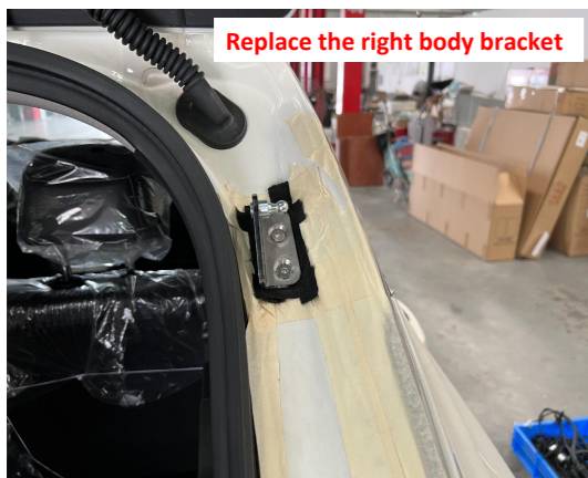
7. Replace the bracket on the right side of the vehicle body.
