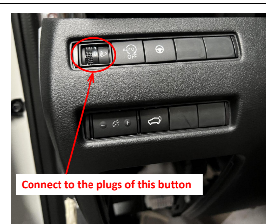
21. Connect to the plugs of the indicated button behind the switch panel.
