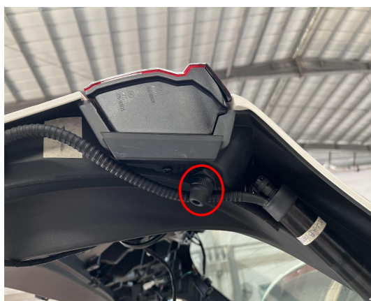
12. Tie the rubber tube of strut wiring harness to the indicated location.
