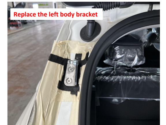
6. Replace the bracket on the left side of the vehicle body.
