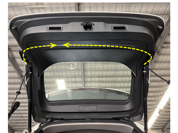
11. Route the strut wiring harnesses as indicated.
