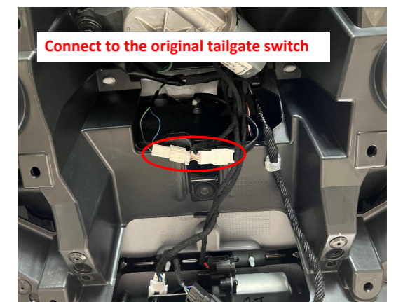
16. Connect the plugs of lock signal harness to original tailgate switch.
