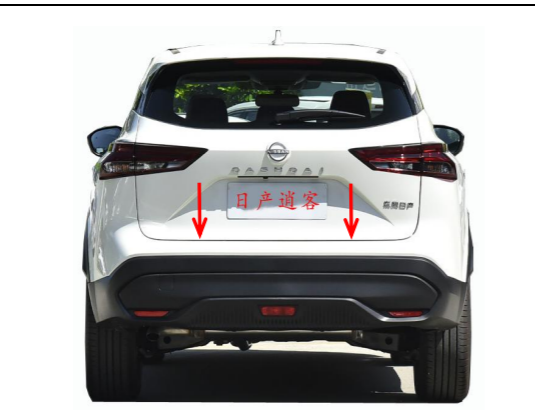
28. Press the added tailgate switch button to open and close the tailgate once for initializing the system, and then test each function of the electric tailgate.
