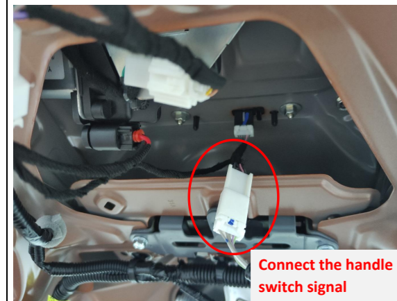
12. Connect the plugs of the lock signal harness to the plugs of the tailgate handle switch.
