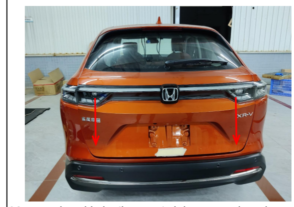
26. Press the added tailgate switch button to close the tailgate once for initializing the system and then test each function of the electric tailgate.
