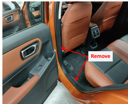
2. Remove the rear left side B-pillar trim panel and door sill panel.
