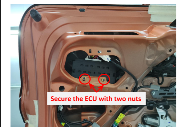
23. Place the ECU at the indicated position and secure it with two nuts.
