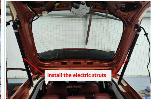
6. Install our electric struts.
