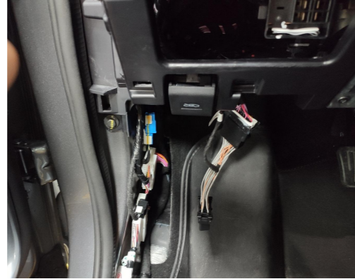
18. Remove the OBD plug from its slot, connect power harness to it, hide the pair of plugs behind the panel and place our OBD plug in the slot of original OBD plug.
