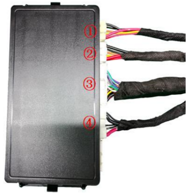
22. Insert the strut wiring harnesses ①②, lock signal harness ③, and power harness ④ into the ECU in sequence.
