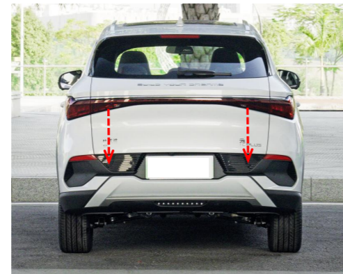
23. Press the added tailgate switch button to open and close the tailgate once for initializing the system, and then test the functions of the electric tailgate.
