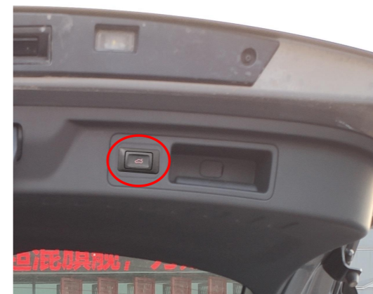
25. Reinstall all trim panels and install the added tailgate switch.
