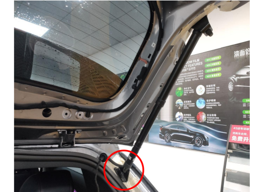
6. Install the electric struts, L on the left and R on the right (the first letter of the strut code), making sure the ends with wiring harnesses are on the vehicle body.
