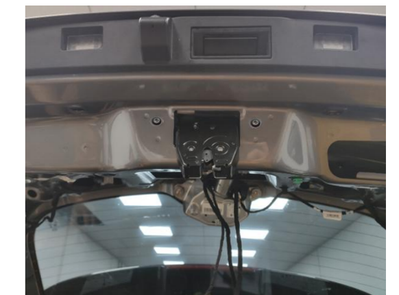
11. Install the power latch and fasten it with provided screws.
