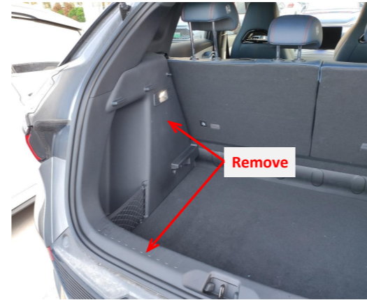
4. Remove the trunk floor mat, door sill panel and the trim panel on the left side of the trunk.
