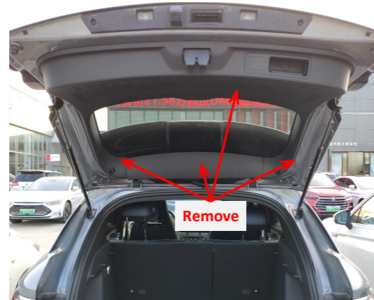
3. Remove the tailgate trim panels.
