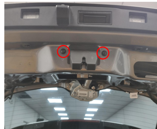
9. Remove the original latch.
