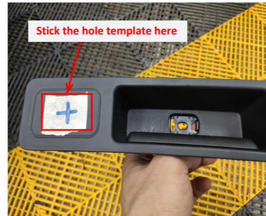
24. Stick the hole template to the indicated position of the handle and open a hole for the added tailgate switch.
