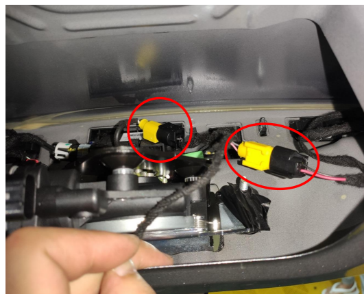
12. Connect the plugs of the lock signal harness to the original tailgate switch behind the power latch.
