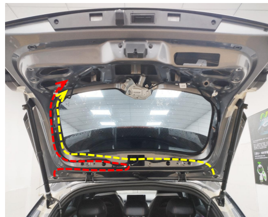
7. Route the left and right strut wiring harnesses to the tailgate.
