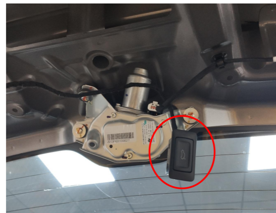
13. Connect the plug of the lock signal harness to the added tailgate switch.
