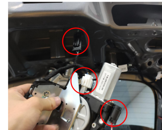
10. Connect the lock signal harness to the plugs of our power latch.
