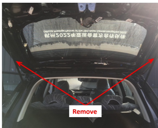
9. Remove the original gas struts.
