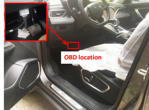
20. Connect the power harness to the OBD plug (connect them inside the trim panel and place the white plug at the slot of the OBD plug).
