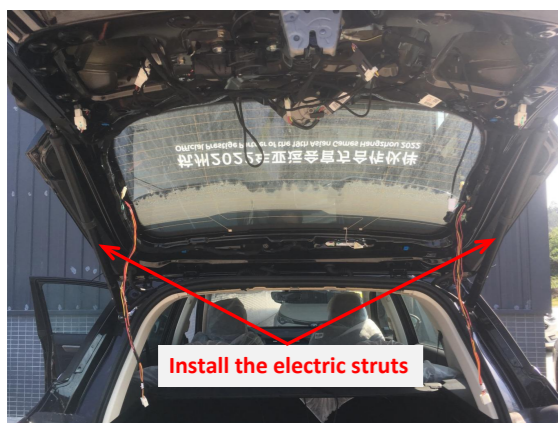
12. Install the electric struts, L on the left and R on the right (the first letter of the strut code).
