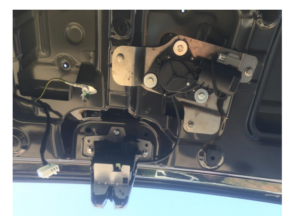
6. Install our latch and actuator.
