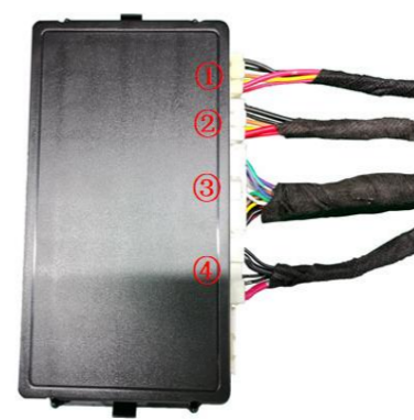
25. Insert the strut wiring harnesses ①②, lock signal harness ③, and power harness ④ into the ECU in sequence.
