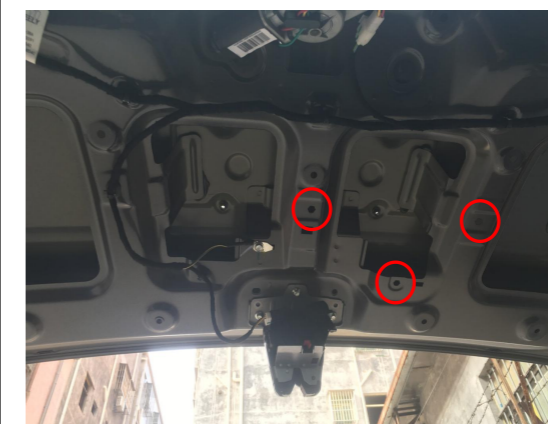
5. Remove the original latch and locate the mounting holes of the lock actuator.
