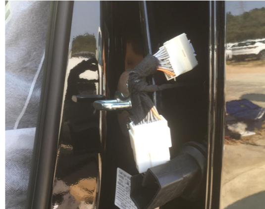
19. Connect the power harness to the B-pillar plugs.
