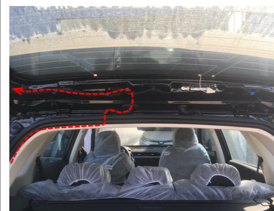
15. Route the power harness to the tailgate (no plug connection before inserting terminals into wiring harness)
