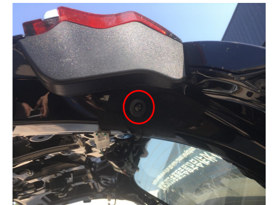
11. Replace the tailgate ball studs.
