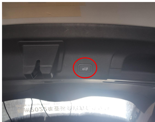
27. Reinstall all trim panels and install the added tailgate switch (remove the small cover panel).
