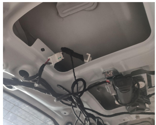
7. Connect the lock signal harness to the plugs of the original tailgate switch button.
