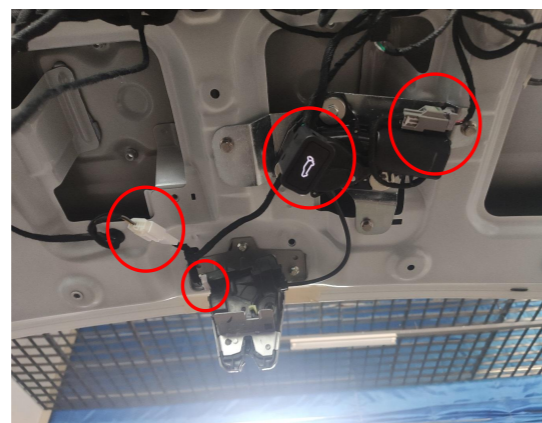
8. Connect the lock signal harness to the plugs of the lock actuator and the added switch.
