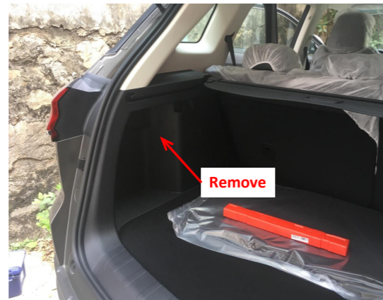
3. Remove the trim panel on the left side of the trunk
