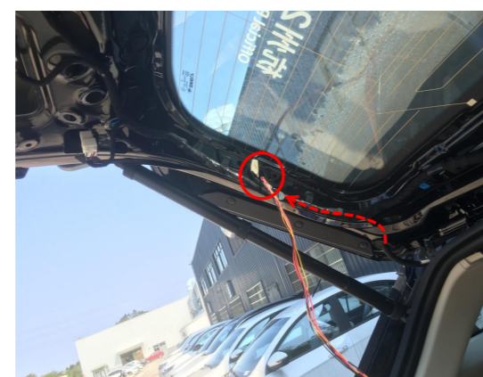
13. Thread the strut wiring harness into the tailgate through the hole on the tailgate.
