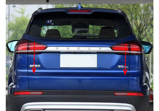
26. Press the added tailgate switch button to open and close the tailgate once for initializing the system, and then test each function of the electric tailgate.
