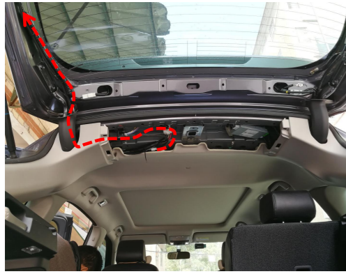
17. Thread the power harness to the tailgate (do not connect plugs before inserting terminals into the wiring harness connector).
