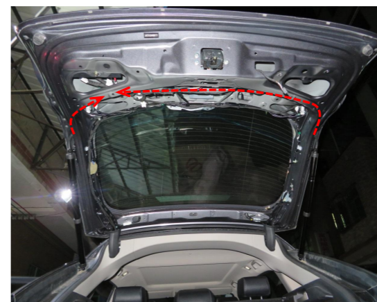
15. Route the strut wiring harnesses.
