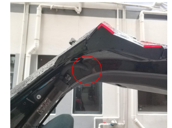
16. Plug the holes on both sides with hole plugs.
