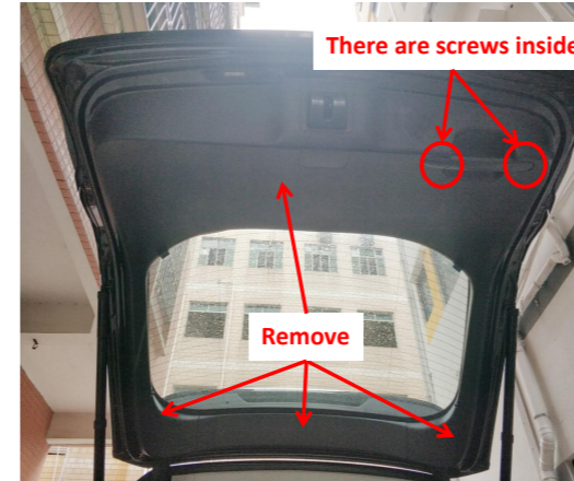
4. Remove the tailgate trim panels.
