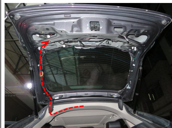
9. Route the lock signal harness.
