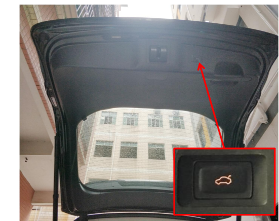
30. Reinstall all trim panels and install the added tailgate switch.
