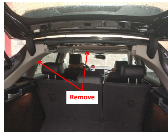
3. Remove the trunk trim panels.
