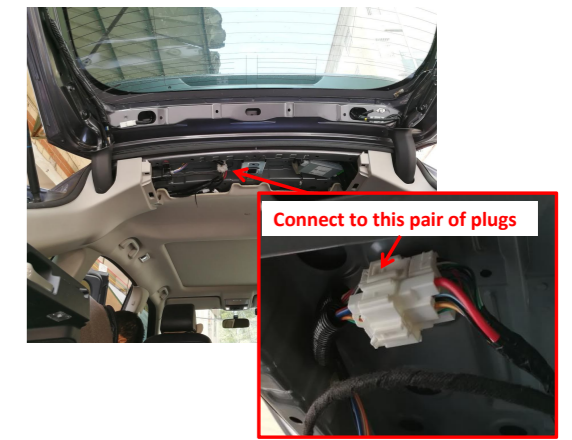
6. Connect the plugs of the lock signal harness to the plugs of the tailgate handle switch.
