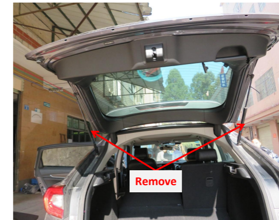
10. Remove the gas struts.
