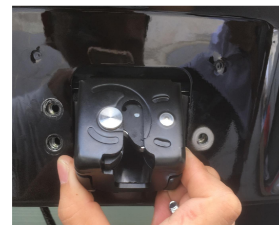
5. Remove the original latch and install our power latch.
