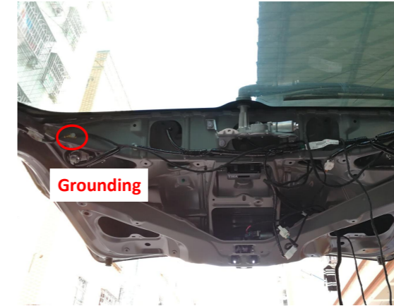
20. Ground at the indicated position.
