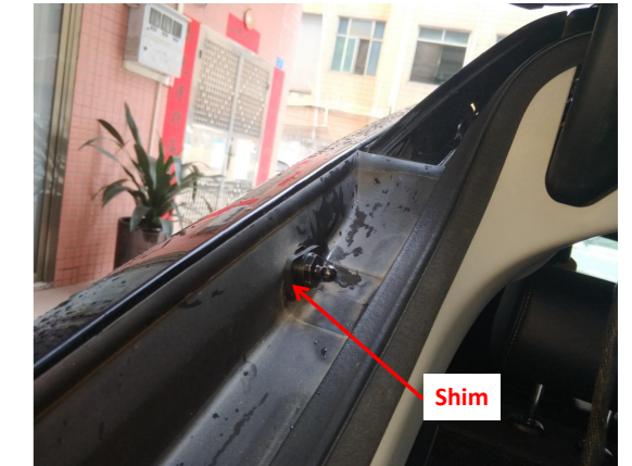
11. Replace the ball stud with our ball studs and shims (both the left and right sides are the same).
