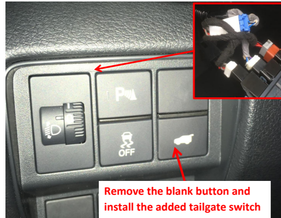
22. Remove the indicated blank button and install the added front switch.
