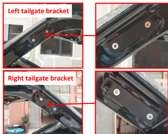
12. Replace the tailgate brackets.
