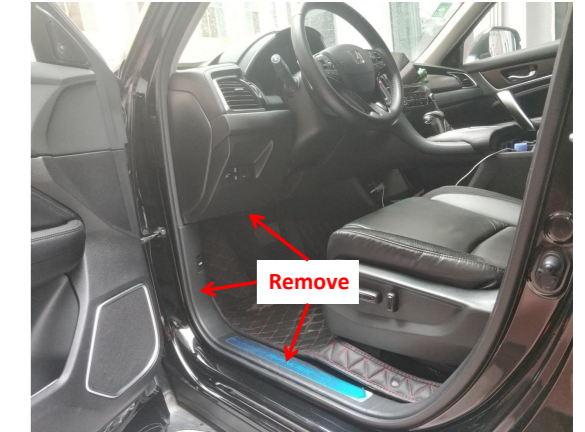
1. Remove the fuse box trim panel under the steering wheel, the front left side trim panel and door sill panel.
