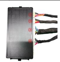
25. Insert the strut wiring harnesses (1)(2), lock signal harness (3), and power harness (4) into the ECU in sequence.
