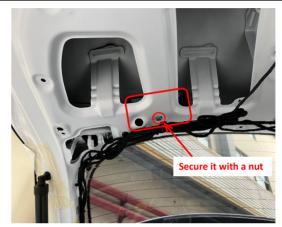
24. Install the ECU and secure it with a nut.
