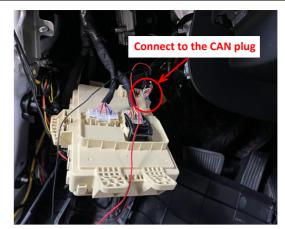
20. Find out the indicated plug and connect the CAN plugs to it and its socket.
