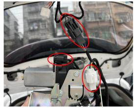
13. Connect the plugs of the lock signal harness with the power latch.
