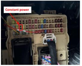
21. The fuse box is located at the driver's area and the fuse slot for power supply is indicated above.
