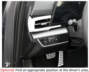
drill a φ21mm hole and install the added front switch.
