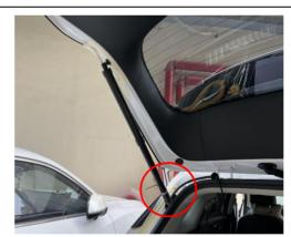
9. Install the electric struts, L on the left and R on the right the first letter of the strut code), making sure the ends with 10. Thread the strut wiring harness through the indicated wiring harnesses are on the car body.
