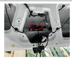
15. Connect the plugs of the lock signal harness to the original tailgate switch outside the tailgate.
