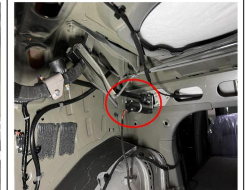
14. Install the left strut (L&R are marked as the first letter of the strut code).
