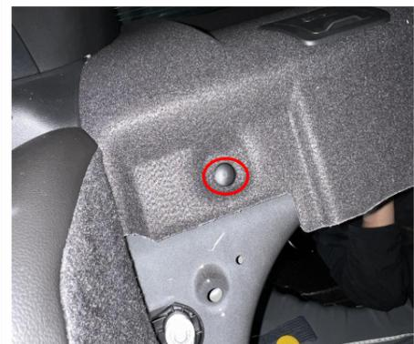
9. Remove the indicated trim panel fastener near the rear seat used to connect with the trunk.
