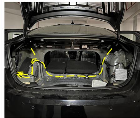
17. Route the left and right strut wiring harnesses to the left side of the trunk along with original wiring harnesses.
