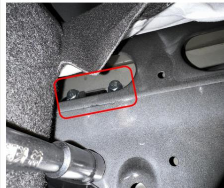
10. Move the edge of the trim panel to reveal the bracket and fasten the nuts.
