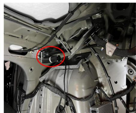
15. Install the left strut (L&R are marked as the first letter of the strut number).
