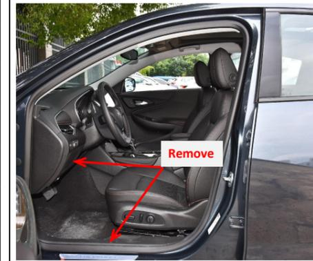
1. Remove the front left door sill panel and fuse box panel.
