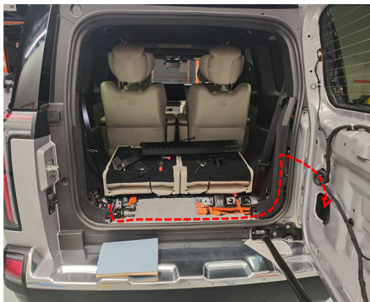
15. Route the power harness to the tailgate as indicated.(no plug connection for now)
