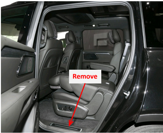
2. Remove the rear left door sill panel.
