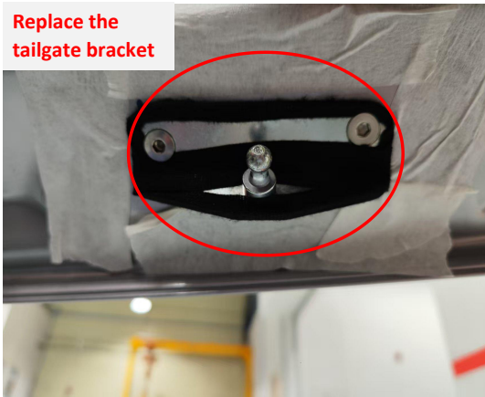
7. Replace the tailgate bracket and use the provided screws.
