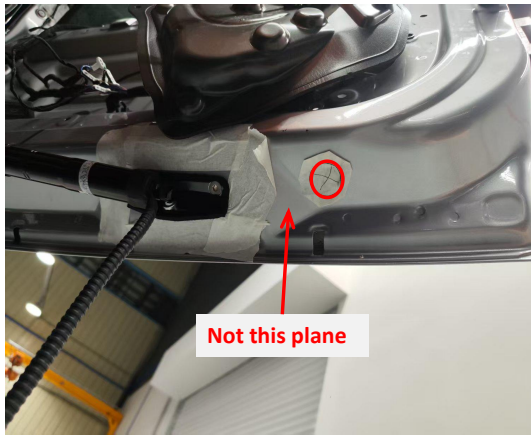
10. Drill a \phi 21\text{mm} hole at the indicated position to allow the strut wire harness to pass through and plug the hole.
