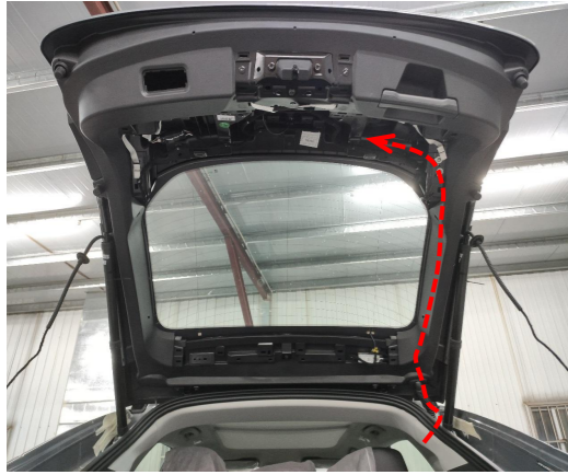
17. Thread the power harness to the tailgate.
