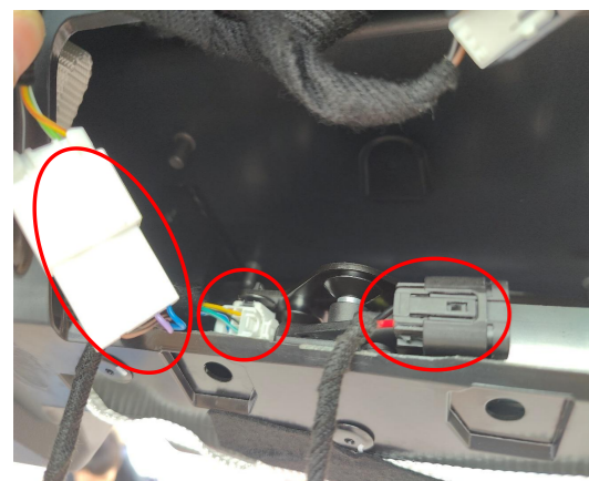
12. Connect the plugs of the lock signal harness to the plugs of the power latch.
