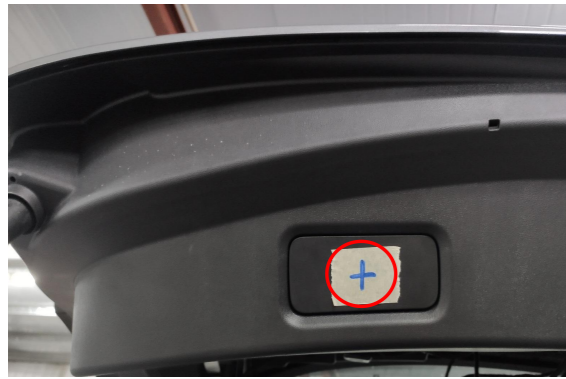
27. Remove the small panel, stick the hole template to it and then drill a hole for the added switch.
