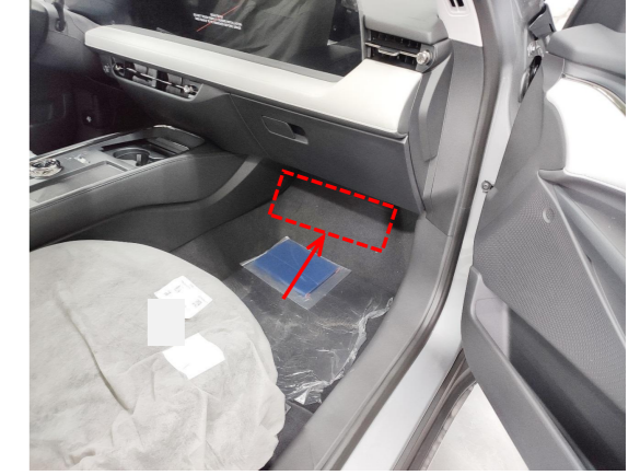
21. The fuse box is located under the storage box of the passenger seat.
