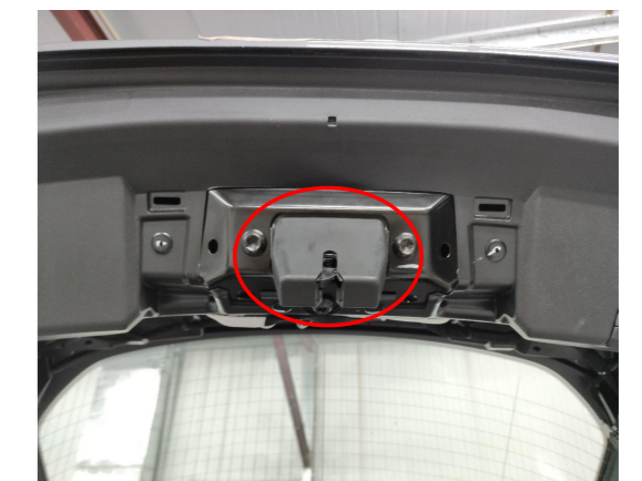
11. Remove the original latch.
