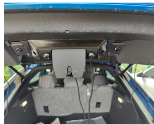
13. Install the power latch.
