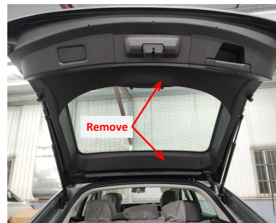
3. Remove the tailgate trim panels.
