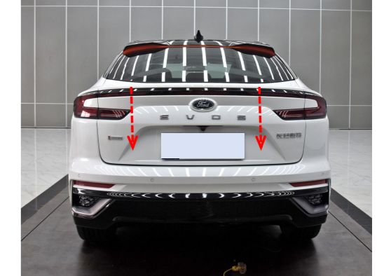
26. Press the added tailgate switch to open and close the tailgate once for initializing the system, and then test each function of the electric tailgate.
