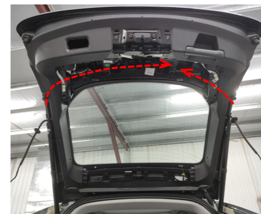
9. Thread the strut wiring harness through the original holes and route the harnesses as shown above.
