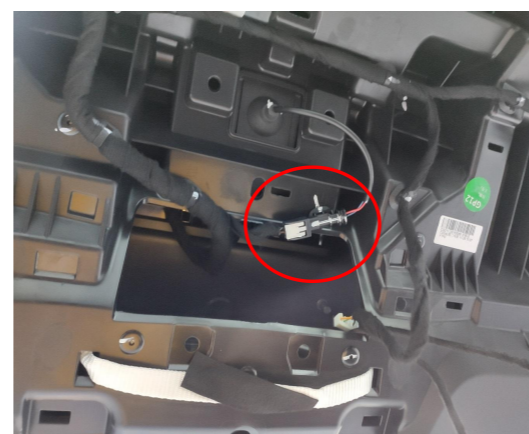
14. Connect the plugs of the lock signal harness to the original tailgate switch.
