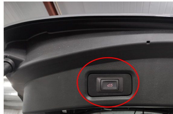
28. Reinstall all trim panels and install the added tailgate switch.
