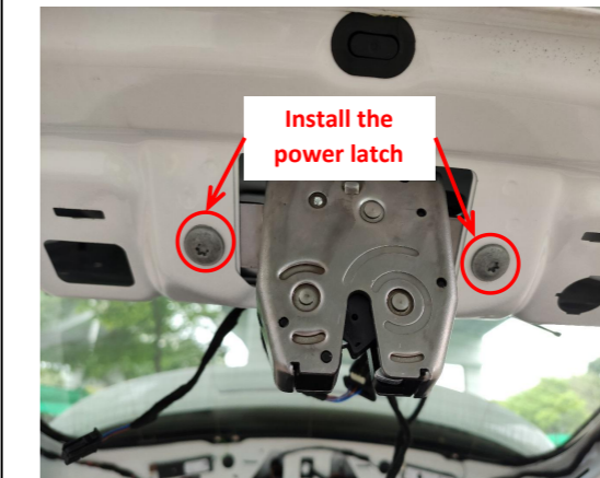
15. Install the power latch.
