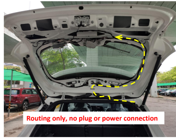
19. Route the power harness to the tailgate.
