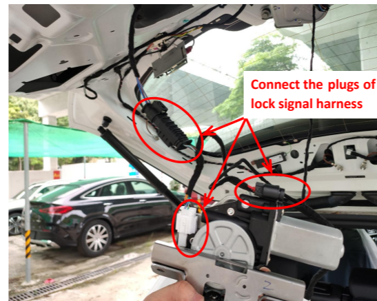
14. Connect the plugs of the lock signal harness to the plugs of the power latch.
