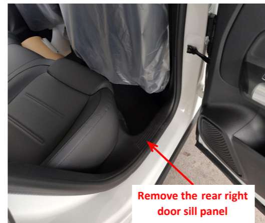
4. Remove the rear right door sill panel.
