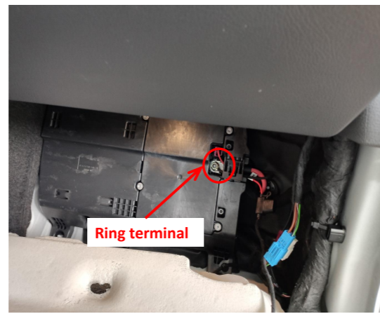
23. Connect the ring terminal to the fuse box for power supply.
