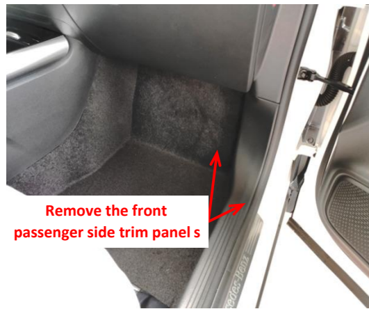
2. Remove the front right side trim panels.
