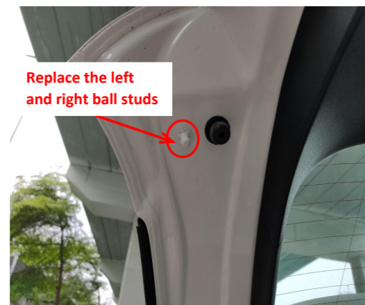
8. Replace the original ball studs on both sides of the tailgate with provided ball studs.
