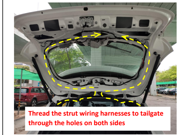
11. Route the left and right strut wiring harness to the tailgate and then connect them to the ECU.
