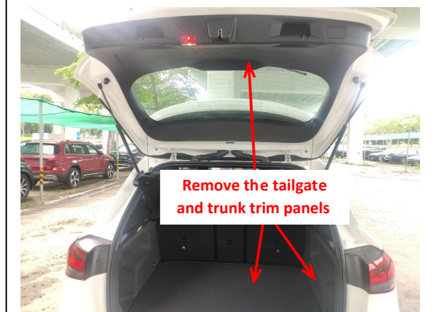
1. Remove the trim panels from the trunk and tailgate.
