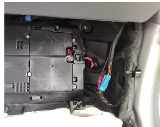
3. Find out the fuse box under the floor mat of front passenger seat.
