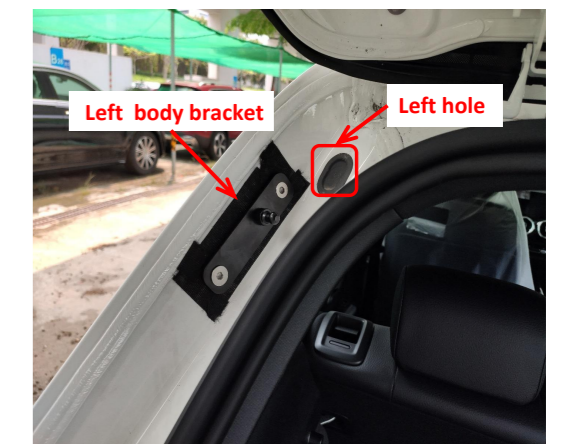
6. Mount the bracket on the left side of car body.
