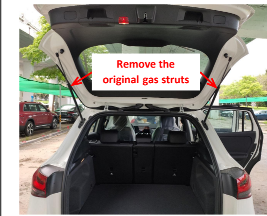
5. Remove the original gas struts.
