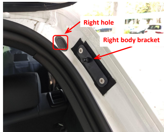
7. Mount the bracket on the right side of the car body.
