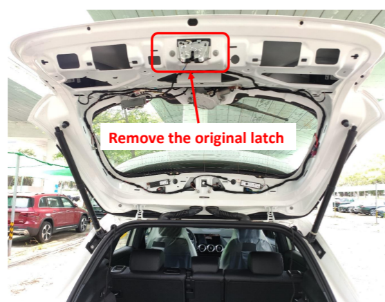
13. Remove the original latch.
