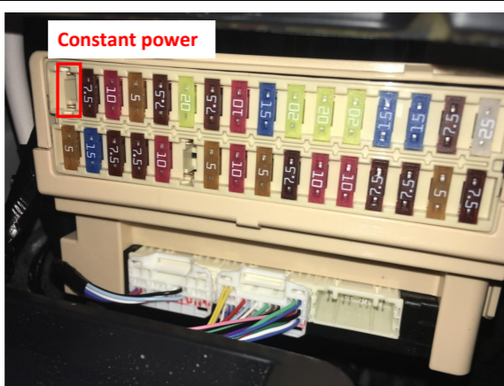
23. The constant power fuse slot (first in the first row).
