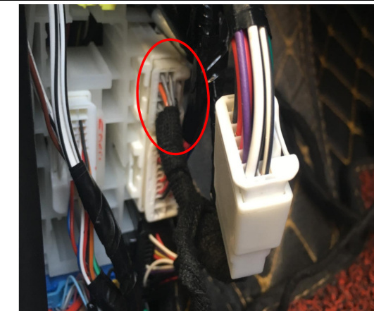
21. Connect the power harness to the signal plug and its socket beside the rest pedal.
