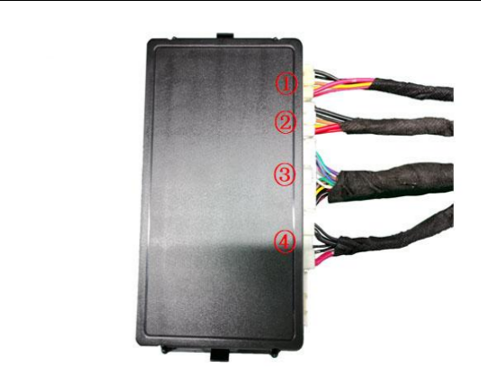
26. Insert the strut wiring harnesses ①②, lock signal harness ③, and power harness ④ into the ECU in sequence, and then mount the ECU onto its bracket.
