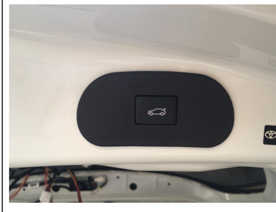
10. Connect the lock signal harness to the added tailgate switch.
