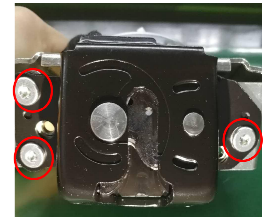
6. Remove the screws from our power latch.
