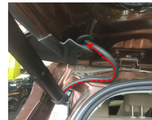
15. Leave a certain length of the rubber tube outside to let it bend at the top of the sink while routing the wiring harness as indicated to prevent it from being squeezed during the tailgate closing process.
