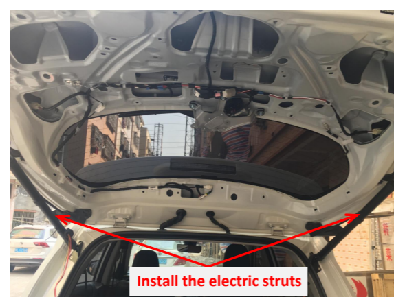
13. Install the electric struts, L on the left and R on the right (the first letter of the strut code).
