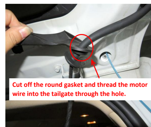
14. Thread the motor wire of strut wiring harness through the hole to the tailgate. Both sides are the same.
