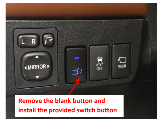
22. Install the provided switch button on the switch panel (connect the plugs for backlight behind the switch panel).
