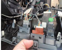
29. Install the added front switch and connect the plugs for backlight.
