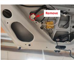
33. Remove the indicated fastener. 34. Install the ECU and secure it with a nut.
