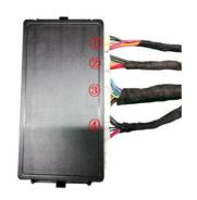
35. Insert the strut wiring harnesses (1)(2), lock signal harness (3), and power harness (4) into the completes initialization and test each function of the ECU in sequence.
