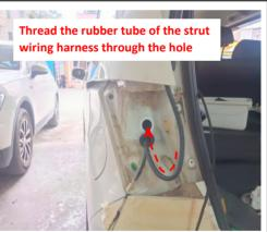
13. Thread the rubber tube of the strut wiring 12. Remove the left and right taillight and remove harness through the hole, both sides are the
