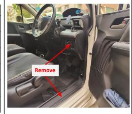
. Remove the front right side door sill panel and . Remove the rear right side door sill panel.
