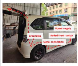
23. Route the power harness (routing only, no olug or power connection).
