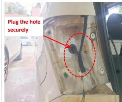
14. Wrap the wiring harness with electric tape and pay attention to avoid pulling it. Plug the holes on both sides securely.
