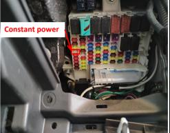
31. The fuse box is located at the driver's position and the fuse slot for power supply is indicated
