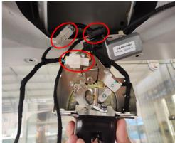
18. Connect the plugs of the lock signal harness to the plugs of the power latch.
