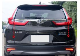
29. Press the added tailgate switch button once to initialize the system once and then test each function of the electric tailgate.
