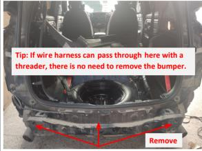
5. Remove the bumpers (if wiring harness can pass through here with a threader, there is no need to remove the
