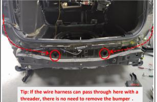
10. Remove the plugs from the holes and thread the strut wiring harnesses through the holes into the car body.
