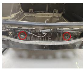
8. Thread the wiring harnesses through the holes of the bumper.
