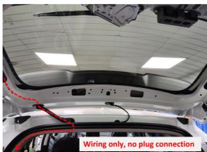
14. Route the lock signal harness to the left side of the trunk.
