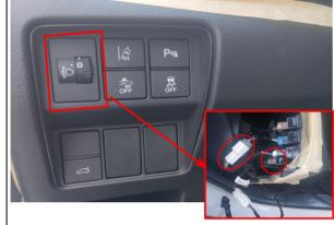
23. Connect the power harness to the plugs of the front switch behind the panel.
