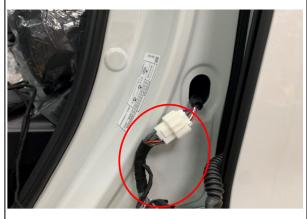
21. Connect the power harness to the indicated plugs at B-
