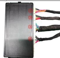
28. Insert the strut wiring harnesses ①②, lock signal harness 3, and power harness 4 into the ECU in sequence and mount the ECU onto its bracket.
