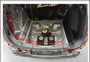
12. Route the strut wiring harnesses to the left side of the trunk.
