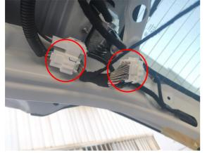
17. Connect the plug of the lock signal harness to the plug of 18. Connect the plugs of the lock signal harness to the plugs of the tailgate handle switch.
