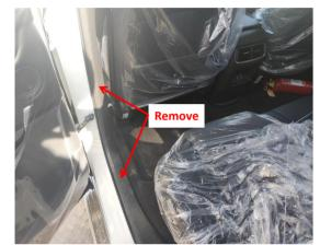
2. Remove the rear left side door sill panel and B-pillar trim
