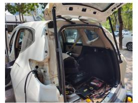
7. Install the electric struts, L on the left R on the right (the first letter of the strut code), making sure the ends with wiring harnesses are on the car body.
