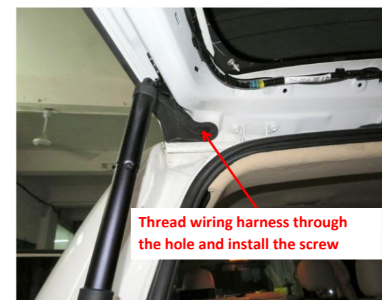
21. Install the screw back and plug the hole tightly. Both sides are the same.
