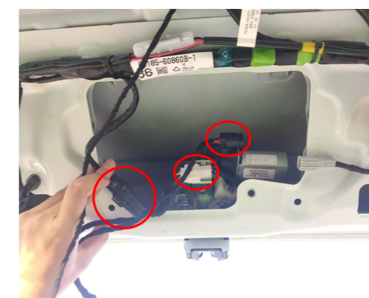
10. Connect the plugs of power latch to the lock signal harness.
