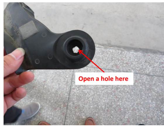
18. Open a hole at the indicated position of the rubber pads (as long as the plugs of strut wiring harness can fit through).
