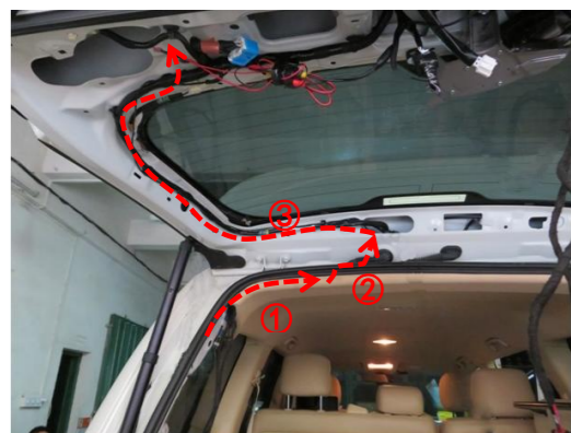
22. Thread the power harness to the left side of tailgate (do not connect plugs before inserting terminals into wiring harness connector).
