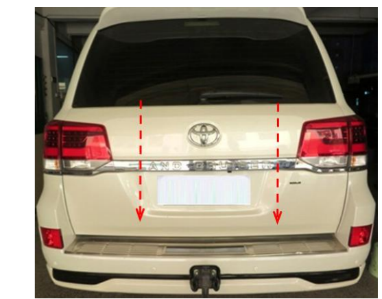
31. Initialize the system once, and then test the functions of the electric tailgate.
