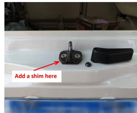
12. Add a shim under the tailgate lock striker (fasten it with the provided screws).
