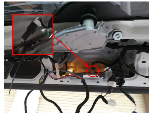
7. Connect the lock signal harness to the handle switch plugs (because the handle switch plugs of the 2016 and 2018 models are different, two pairs of plugs are reserved. Please choose the correct one pair according to the year).
