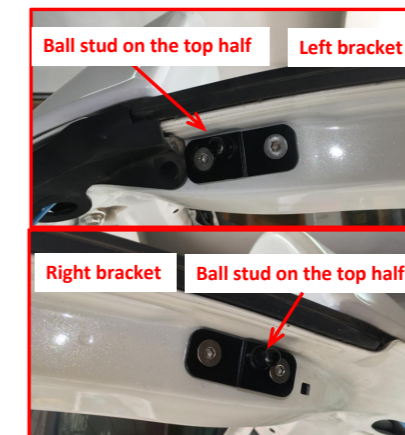
15. Replace the left and right tailgate brackets (the ball studs are on the top half and near the spoiler).
