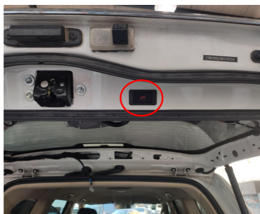
34. Reinstall all the trim panels and install the added tailgate switch.
