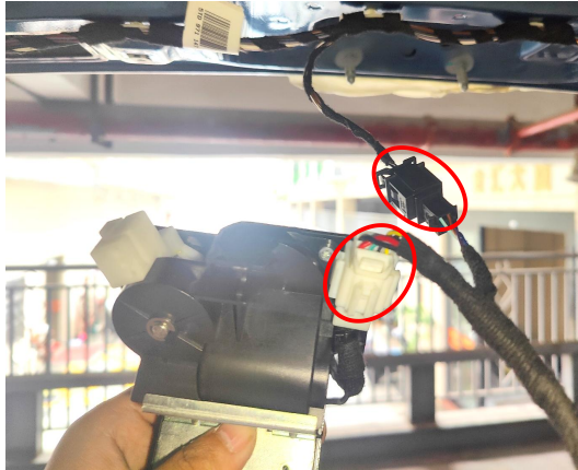
5. Connect the plugs of the lock signal harness to the plugs of the power latch.
