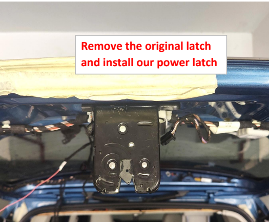
7. Remove the original latch and install our power latch.
