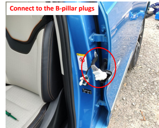
20. Connect the power harness to the B-pillar plugs at the rear left side B-pillar.
