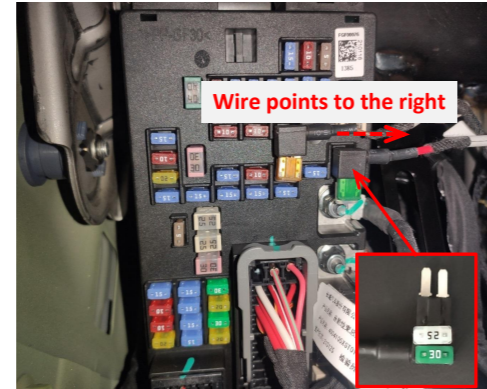
23. Move the fuse from the fuse box to the fuse tap and then plug the fuse tap into the fuse box. Pay attention to the direction.
