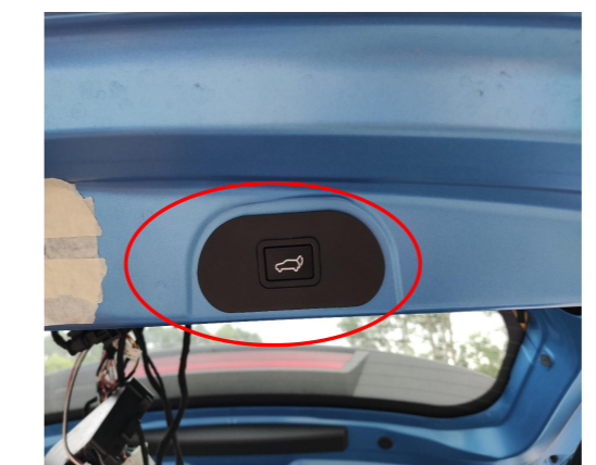
15. Connect the plugs of the lock signal harness to the added tailgate switch.
