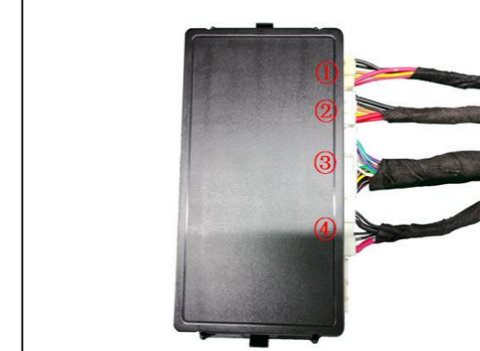
25. Insert the strut wiring harnesses ①②, lock signal harness ③, and power harness ④ into the ECU in sequence.
