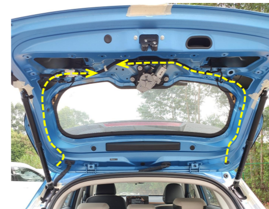
10. Thread the strut wiring harnesses through holes into the tailgate and route them as shown above.
