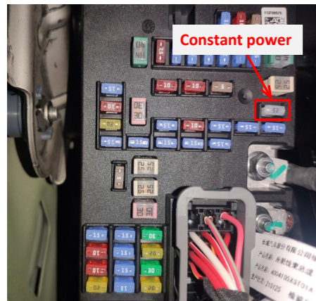
22. The fuse box is located at the driver's area and the fuse slot for power supply is indicated above.
