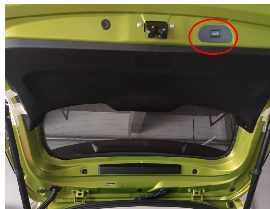
27. Reinstall all trim panels and install the added tailgate switch (remove the original small cover panel).
