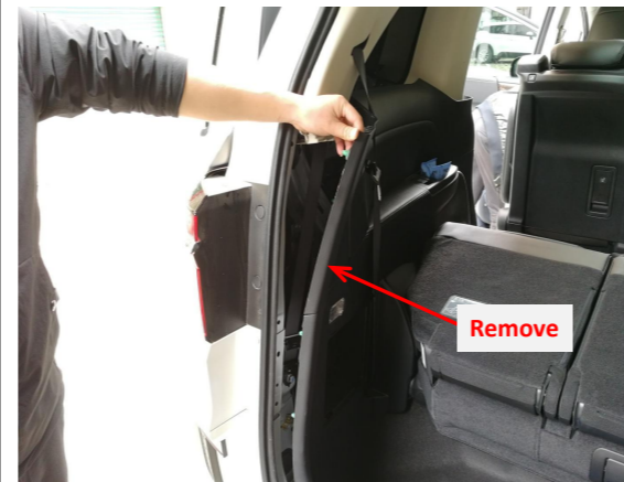
4. Remove the trim panel on the left side of the trunk to allow the wiring harnesses to pass through.
