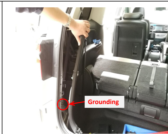
18. Ground at the indicated location on the left side of the trunk.
