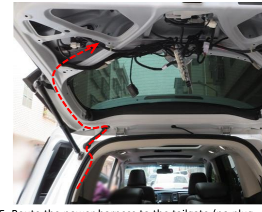
15. Route the power harness to the tailgate (no plug connection before inserting terminals into the wiring harness connector).
