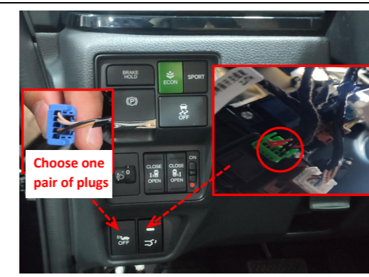
20. Remove the blank button, install the added front switch and connect the plugs for backlight behind the panel (due to configuration differences, several pairs of plugs have been reserved. Choose the correct one pair for connection).
