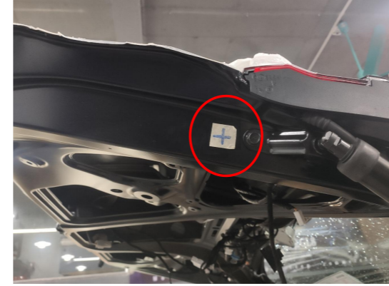
9. Use a \phi 21\text{mm} drill bit to drill a hole at the indicated position to allow the strut wiring harness to pass through. Both the left and right sides follow the same method.
