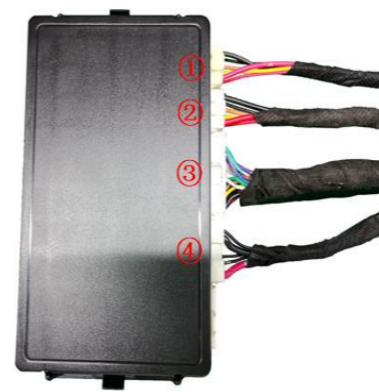
24. Insert the strut wiring harnesses ①②, lock signal harness ③, and power harness ④ into the ECU in sequence and mount the ECU onto its bracket.
