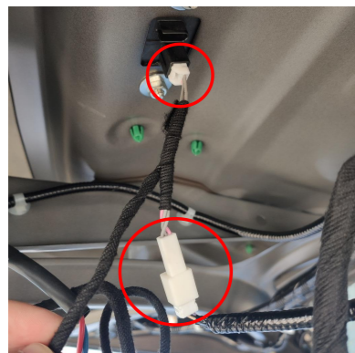
12. Connect the plugs of the lock signal harness to the plugs of the original tailgate switch.
