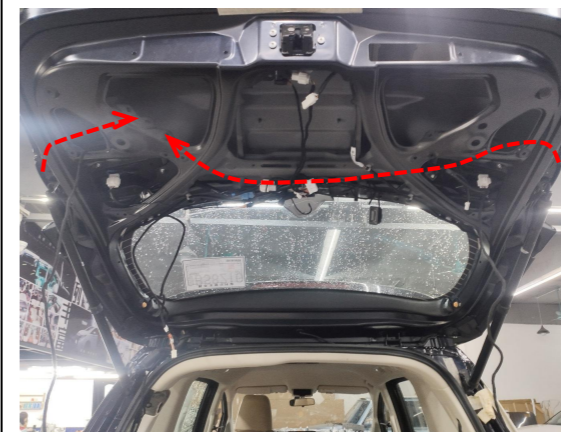
10. Route the strut wiring harnesses and then plug the holes with hole plugs.
