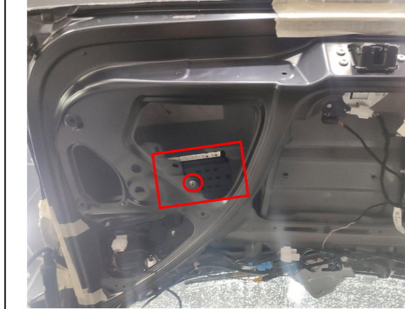
23. Place the ECU bracket at the indicated position and secure it with a nut.
