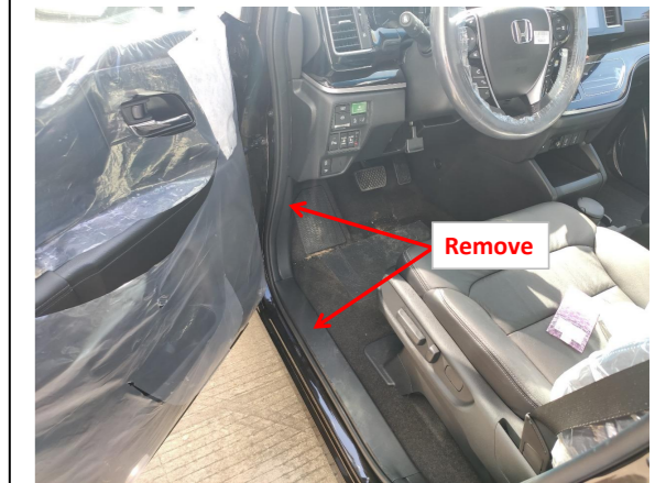
1. Remove the front the side trim panel and door sill panel.
