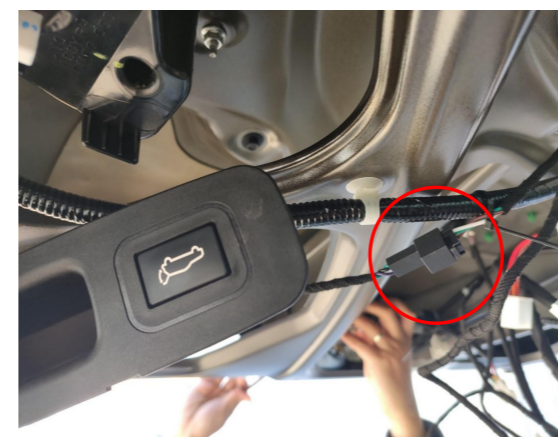
14. Connect the plug of the lock signal harness to the added tailgate switch.
