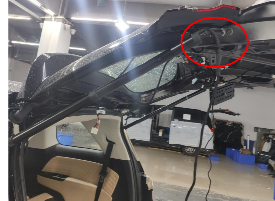
8. Install the electric struts, L on the left and R on the right (the first letter of the strut code), making sure the ends with wiring harnesses are on the tailgate.
