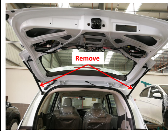
5. Remove the gas struts.
