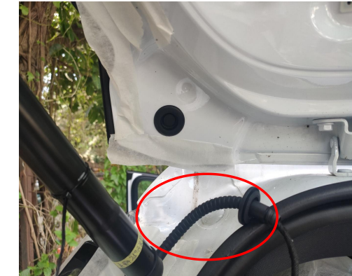
6. Install the electric struts, L on the left and R on the right (the first letter of the strut number), making sure the ends with wiring harnesses are on the vehicle body.
