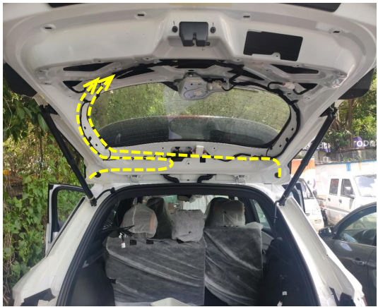
8. Route the strut wiring harnesses to the tailgate.
