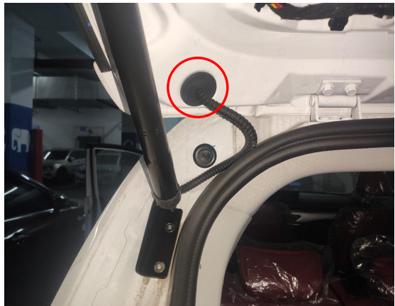
10. Plug the holes on both sides securely.
