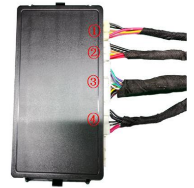
26. Insert the strut wiring harnesses ①②, lock signal harness ③, and power harness ④ into the ECU in sequence.
