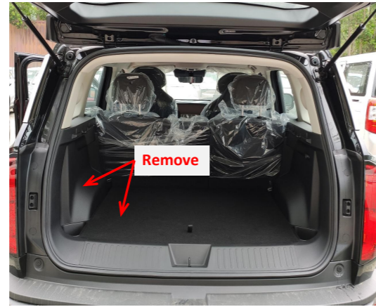
3. Remove the trunk floor mat and left side trim panel.
