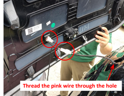
13. Connect the lock signal harness to the plugs of original tailgate switch, thread the pink wire through the indicated hole into tailgate and then reinstall the trim panel.
