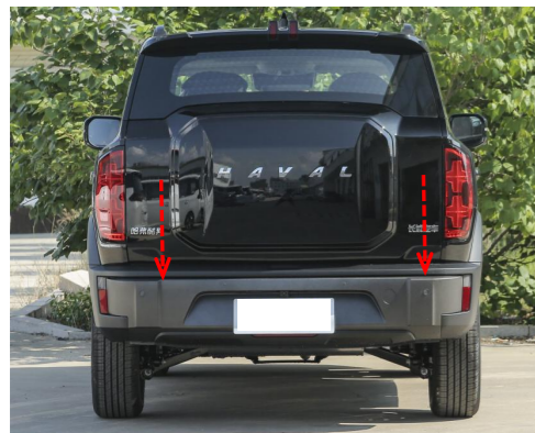
27. Press the added tailgate switch button to open and close the tailgate once for initializing the system, and then test each function of the electric tailgate.
