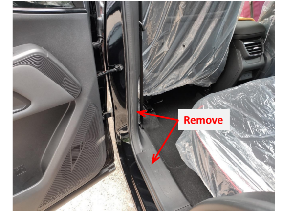
1. Remove the rear left side door sill panel and B-pillar trim panel.
