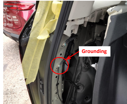
19. Ground at the right side of the tailgate.
