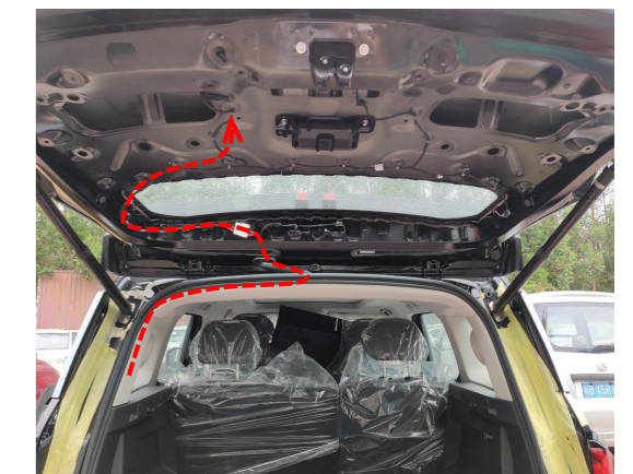
16. Thread power harness to the tailgate (wiring only, no plug or power connection).
