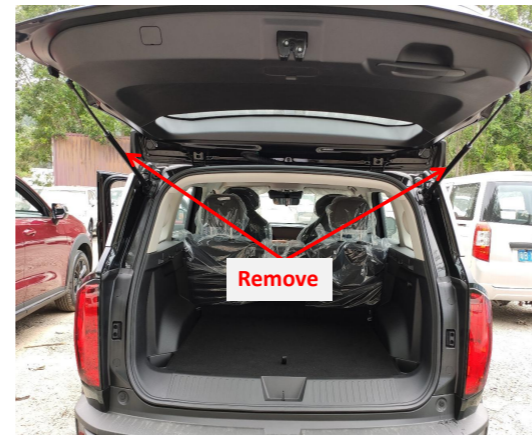
4. Remove the original gas struts.
