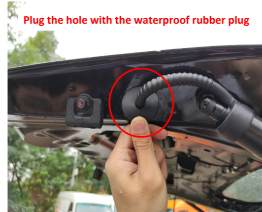
9. Plug the hole with the waterproof plug securely.
