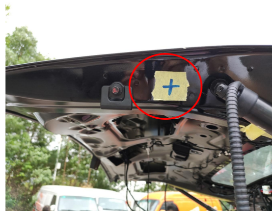
8. Drill a hole at the indicated position on the tailgate with a \phi 21\text{mm} drill bit; both sides are the same.
