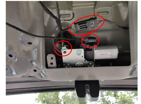
11. Connect the lock signal harness to the plugs of the power latch.
