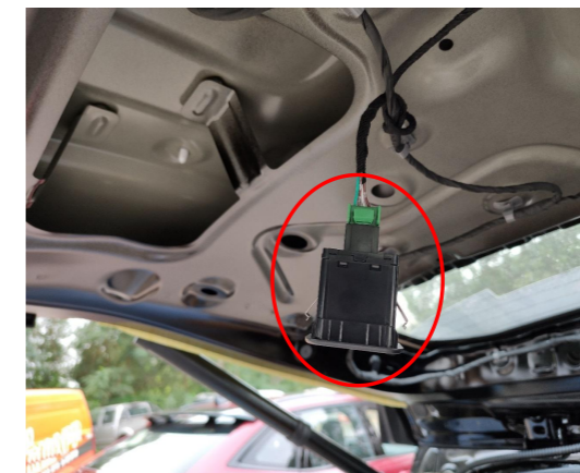
15. Connect the lock signal harness to the added tailgate switch.
