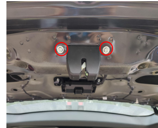
10. Replace the original latch with our power latch.
