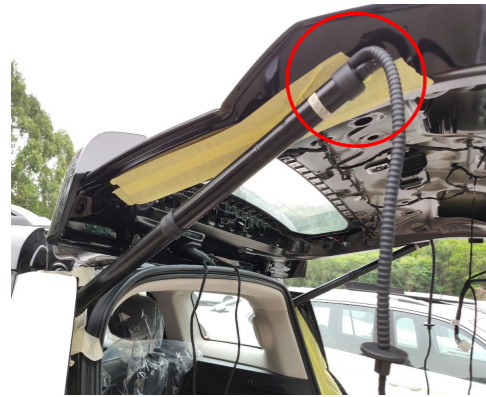
7. Install the electric struts, L on the left and R on the right (the first letter of the strut code), making sure the ends with wiring harnesses are on the tailgate.
