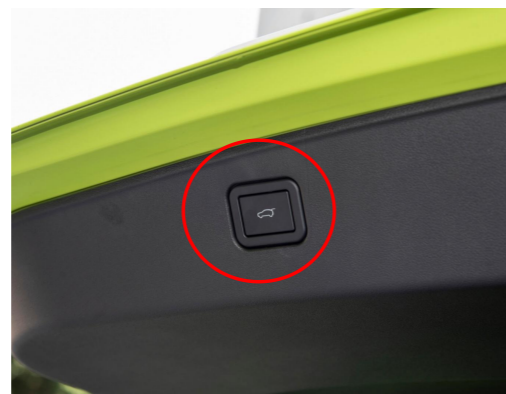
28. Reinstall all trim panels and install the added tailgate switch (remove the original small cover panel).
