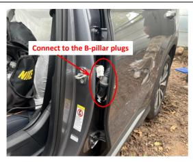
18. Connect to the B-pillar plugs at rear left B-pillar.
