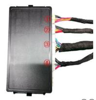
23Insert the left and right strut wiring harnesses (1)(2), lock 24. Press the added tailgate switch to close the tailgate signal harness (3), and power harness (4) into the ECU in sequence.
