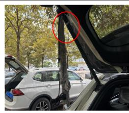
8. Install the electric struts, L on the left and R on the right the first letter of the strut code).
