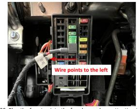
20. Plug the fuse tap into the fuse box and pay attention to the direction of wire.
