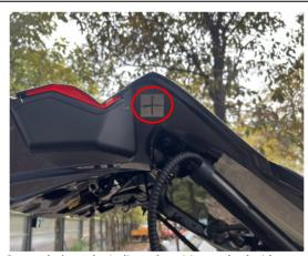
Open a hole at the indicated position on both sides to allow the wiring harnesses to pass through.
