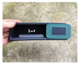
25. Stick the hole template to the indicated position of the tailgate handle and open a hole for the added tailgate
