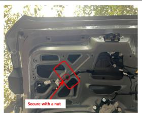
22. Install the ECU and secure it with a nut.
