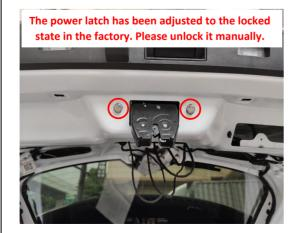
13. Install the power latch with provided screws.
