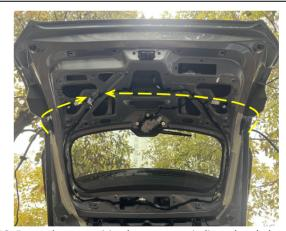
10. Route the strut wiring harnesses as indicated and plug the holes with the rubber plugs.
