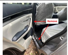
2. Remove the rear left door sill panel and B-pillar trim
