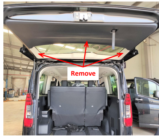
2. Remove the tailgate trim panels.
