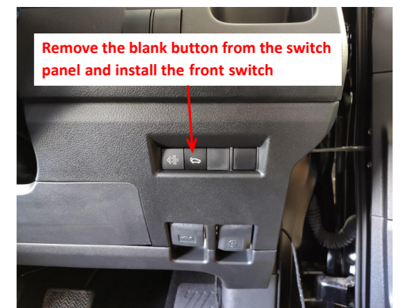
21. Remove the blank button from the switch panel and install the added front switch.
