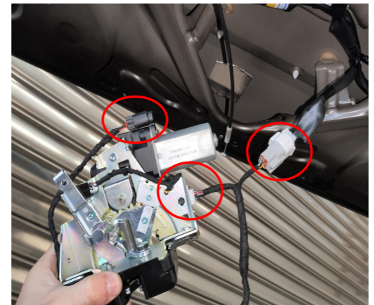
13. Connect the lock signal harness to the plugs of the power latch.
