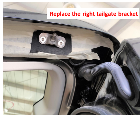
8. Replace the right tailgate bracket.
