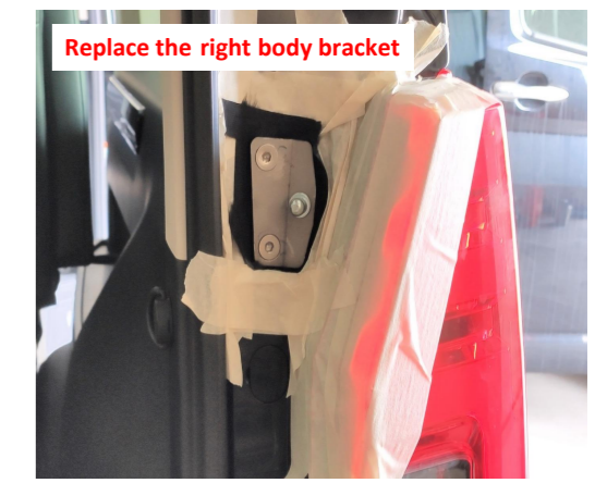
6. Replace the right body bracket.
