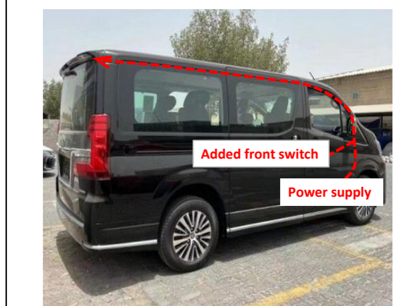
16. Route the power harness through the roof (routing only, no plug or power connection).
