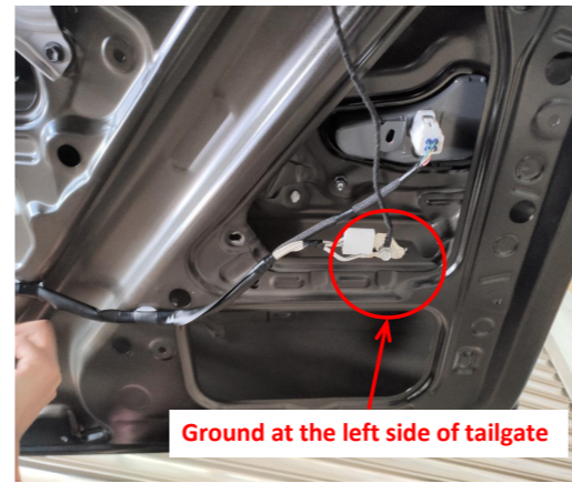
19. Ground at the left side of tailgate.
