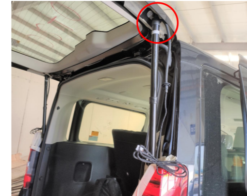
9. Install the electric struts, L on the left and R on the right (the first letter of the strut code), making sure the ends with wiring harnesses are on the tailgate.
