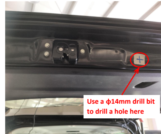
30. Drill a hole at the shown position of the tailgate using a φ14mm drill bit.
