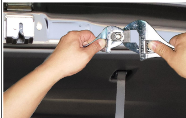
32. Use the wrenches to open the hole.
