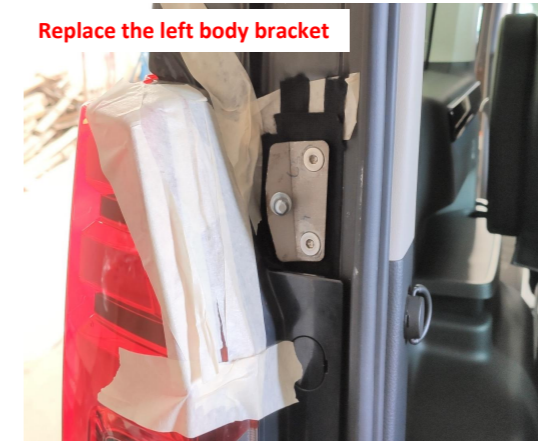
5. Replace the left body bracket.
