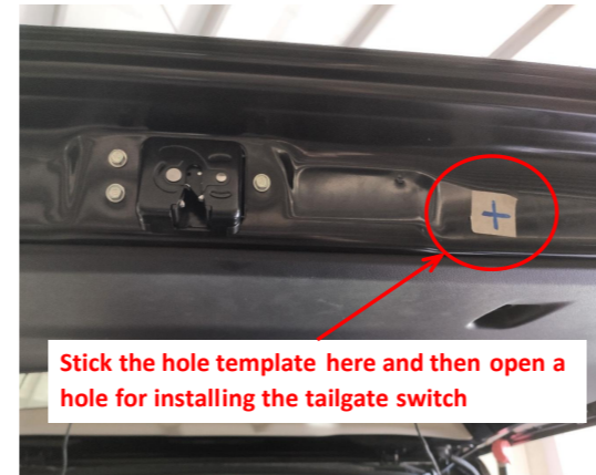
29. Stick the hole template to the indicated position of the tailgate and open a hole for installing the tailgate switch.
