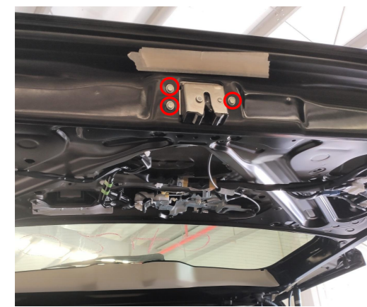
12. Remove the original latch.
