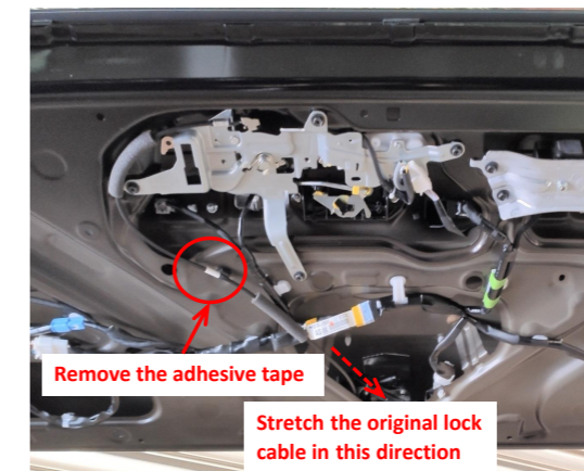
15. Stretch the original lock cable in the direction indicated above for easy installation of the power latch.
