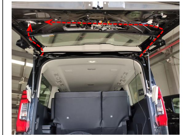
11. Route the left and right strut wiring harnesses to the tailgate.
