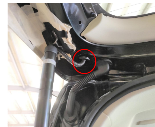
10. Thread the strut wiring harness through the indicated car hole; the same on both sides.
