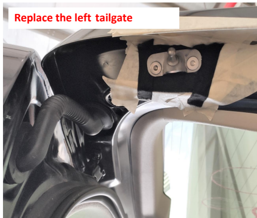
7. Replace the left tailgate bracket.
