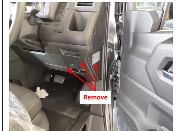
1. Remove the front right side trim panel and switch panel.
