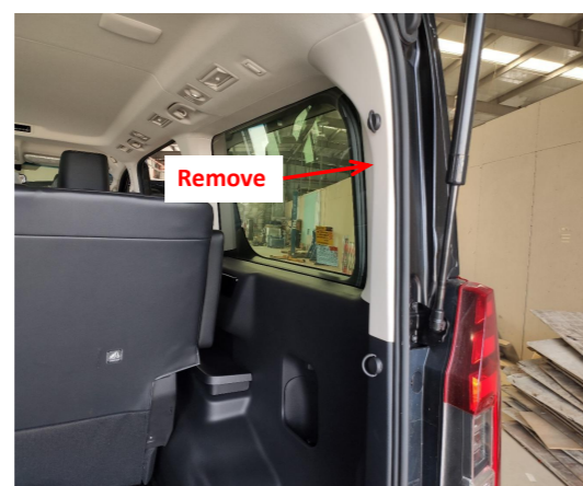
3. Remove the indicated trim panel to allow wiring harnesses to pass through.
