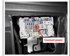
28. The fuse box is located at the left side of the pedals and the fuse slot for power supply is indicated above.
