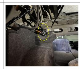
32. Install the trim panels on the left and right sides inside the trunk and properly cut a part of the panel to avoid interference with the operation of the struts.
