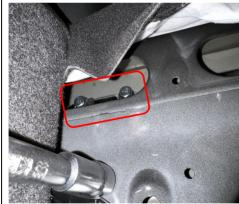
10. Move the edge of the trim panel to reveal the bracket and fasten the nuts.
