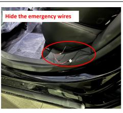
22. Wrap the two emergency wires with electrical tape separately and hide them under the trim panel beside the rear left seat
