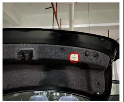
35. Stick the hole template the indicated location and open a hole for the added tailgate switch (as close to the ower edge as possible).
