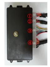
31. Insert the strut wiring harnesses (1)(2), lock signal harness 3, and power harness 4 into the ECU in sequence.
