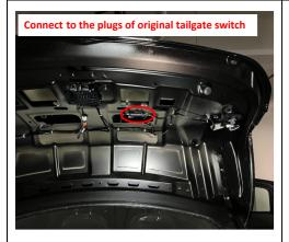
21. Connect the plugs of the lock signal harness to the plugs of original tailgate switch.
