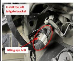
12. Install the provided bolt with bump stop and the lifting eye bolt, pass the M6 bolt through the hole of the 13. Install the right tailgate bracket in the same way. eye bolt and secure them with nuts.
