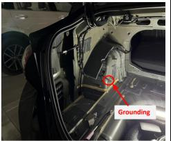
passenger seat and connect the plugs of power harness 25. Ground at indicated location. to the unlock signal plugs.
