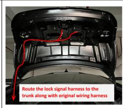
23. Route the lock signal harness to the trunk along with the original wiring harness.
