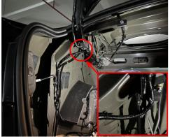
16. Pay attention to keep the struts above the original wiring harnesses to prevent breakage of the wiring harnesses.
