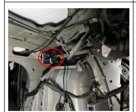
15. Install the left strut (L&R are marked as the first etter of the strut number).
