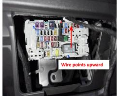
29. Plug the fuse tap into the fuse box. Pay attention to the direction.
