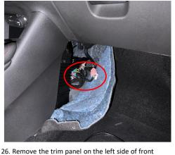
Check if all the plugs are well connected; Use original emergency key to make sure whether the latch can be unlock normally, and check whether the emergency wires are properly installed.
