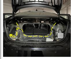
17. Route the left and right strut wiring harnesses to the left side of the trunk along with original wiring harnesses.
