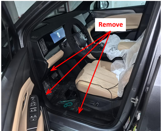
1. Remove the front left side door sill panels and the trim panel of the fuse box.
