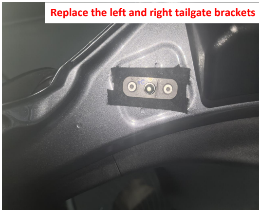
8. Replace the left and right tailgate brackets.
