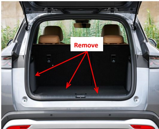
3. Remove the trim panel on the left side of the trunk, the floor mat and the foam storage box.
