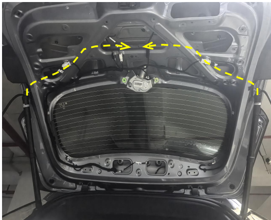
11. Route the strut wiring harnesses as indicated.
