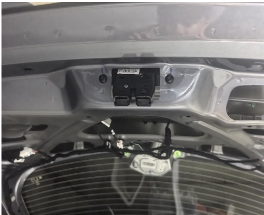
12. Remove the original latch.
