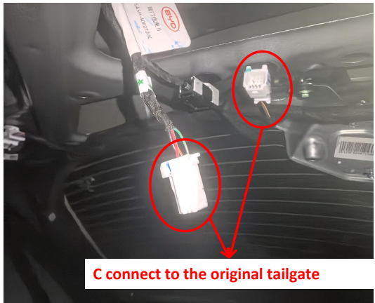
15. Connect the plugs of the lock signal harness to the plugs of original tailgate switch.
