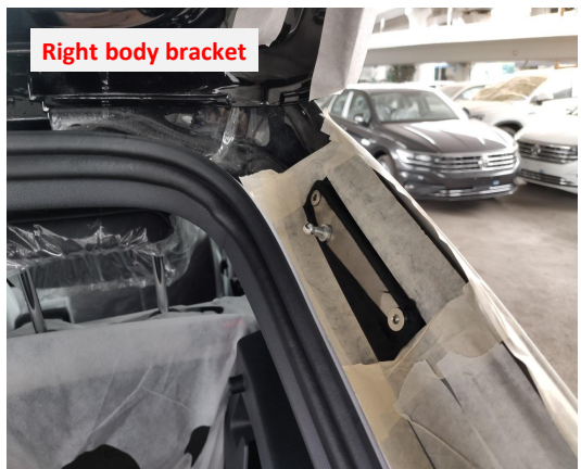
8. Replace the right body bracket.
