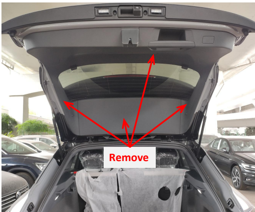
4. Remove the tailgate trim panels.
