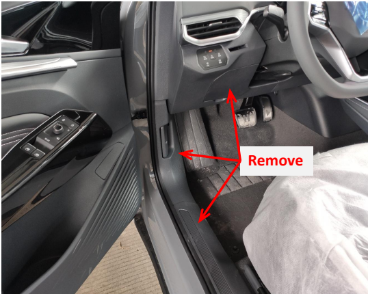
1. Remove the front left side trim panel and door sill panel.
