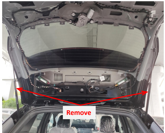
6. Remove the original gas struts.
