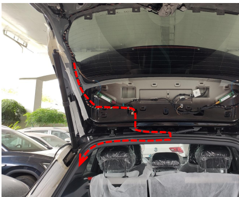
16. Route the lock signal harness to the left side of the trunk (no plug connection before inserting terminals into the wiring connector).
