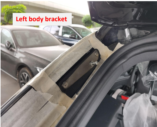
7. Replace the Left body bracket.
