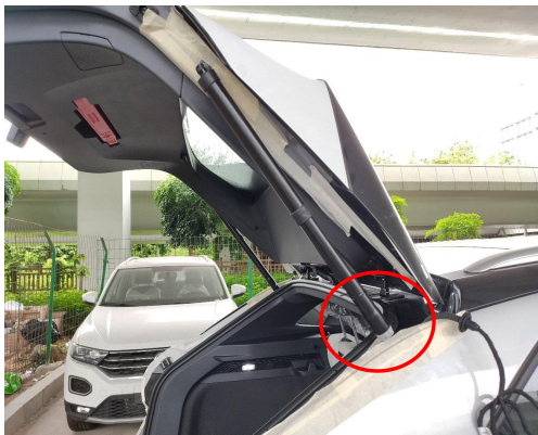
9. Install the electric struts, L on the left and R on the right (the first letter of the strut code), making sure the ends with wirings are on the car body.
