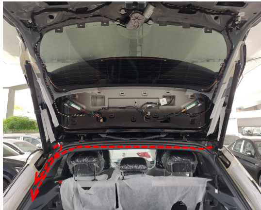
11. Route the strut wiring harnesses to the left side of the trunk.
