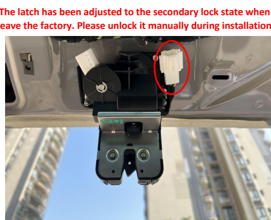
15. Install the power latch and fix the indicated plug to it's original position.
