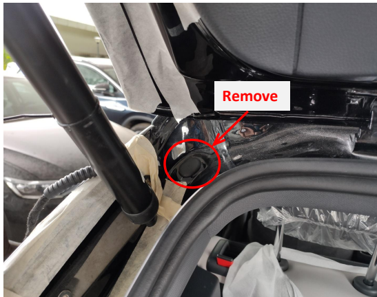
10. Remove the rubber plug from the hole to allow the strut wiring to pass through; both sides are the same.
