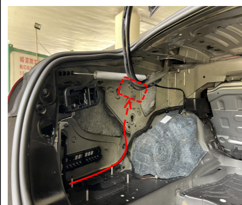
18. Route the left and right strut wiring harness to the location of the ECU.
