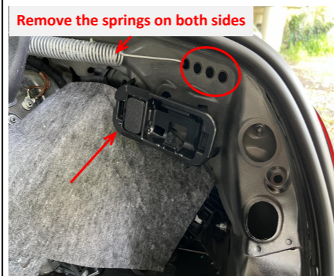
5. Remove the springs on both sides. Install the right body bracket at the indicated holes and insert the screw with handle into the body from the indicated direction.
