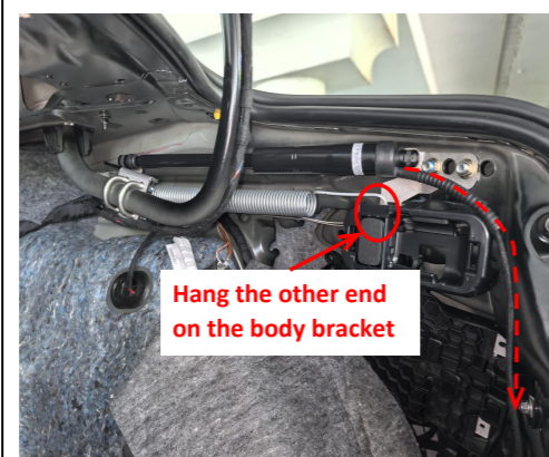
16. Install the electric struts, L on the left and R on the right (the first letter of the strut code). Pay attention to the direction of the wiring harness.
