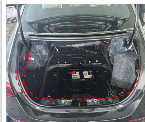
17. Route the left and right strut wiring harness to the left side of the trunk along with the original wiring harness.
