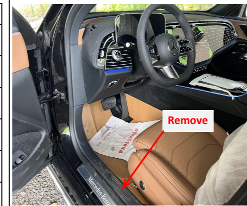
1. Remove the front left side door sill panel.
