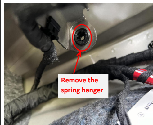
10. Remove the springs hangers on the left and right hinges.
