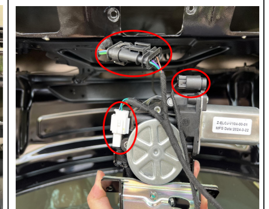
20. Connect the plugs of the lock signal harness to the plugs of the power latch.
