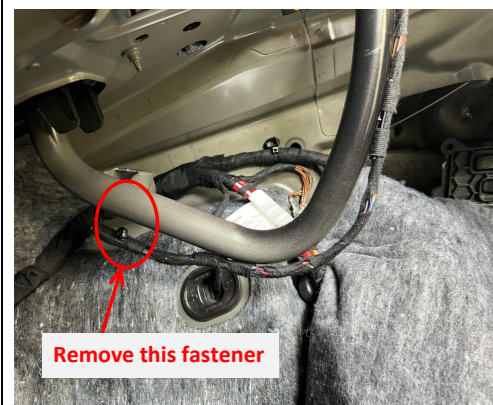
9. Remove the indicated fasteners on both sides.
