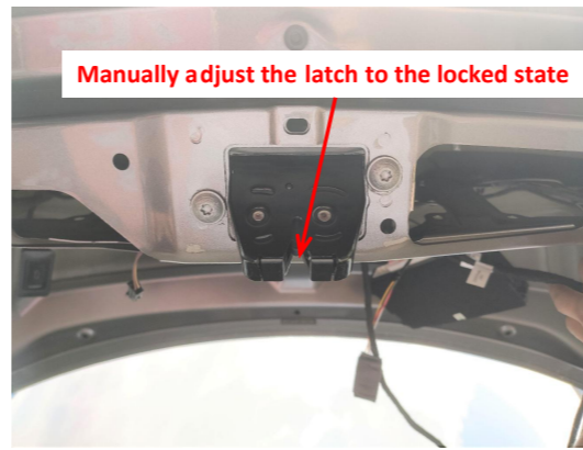
19. Install the power latch and manually adjust the latch to the locked state to prevent accidental closing during installation process.
