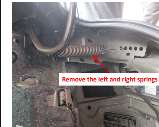
5. Remove the original springs from the both sides of the trunk.
