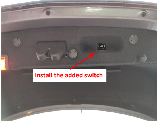
32. Reinstall all the trim panels and install the added tailgate switch.
