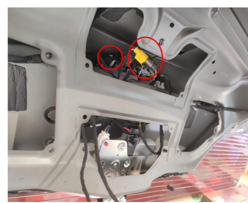
20. Connect the plugs of the lock signal harness to the plugs of the original tailgate switch and the added tailgate switch.
