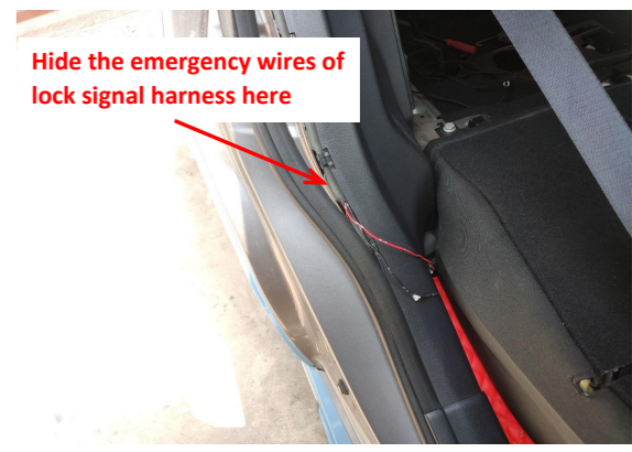
21. Route the emergency wires of the lock signal harness along the right hinge to the right side of rear seat (the emergency wires should be in place for emergency use).
