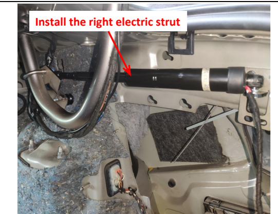
12. Install the right electric strut, L on the left and R on the right (the first letter of the strut code), making sure the end with wiring harness points outward.
