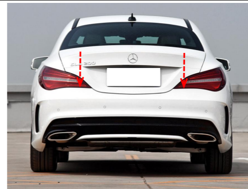
30. Manually close the tailgate until it touches the striker, then press the original tailgate switch button to open the tailgate. The system will complete initialization, and then test each function of the electric tailgate.
