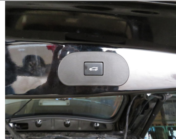
8. Install the added tailgate switch at the tailgate handle.
