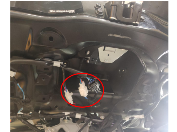
6. Connect lock signal harness to the plugs of the power latch.
