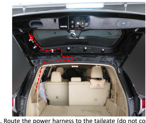
15. Route the power harness to the tailgate (do not connect power before inserting terminals into the wiring harness connector).
