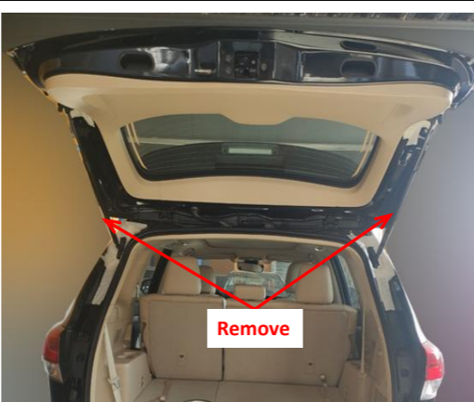
9. Remove the gas struts.
