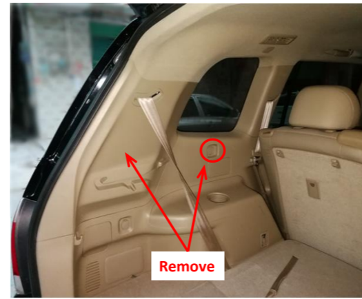
4. Remove the trim panel on the left side of the trunk (there are screws in the circle).
