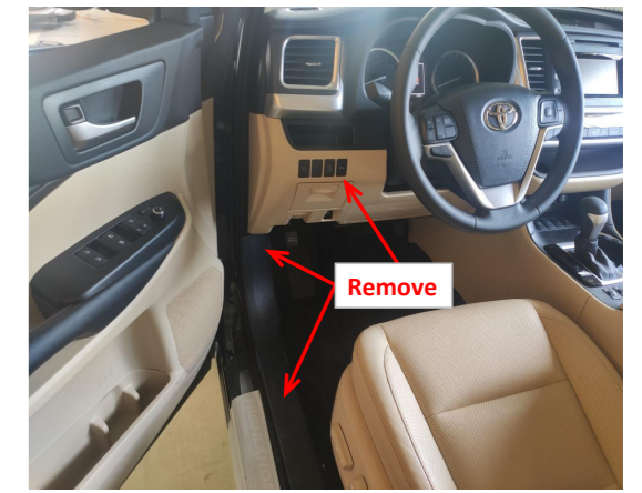
1. Remove the front left side trim panel and door sill panels.
