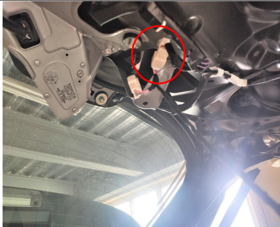
7. Connect the lock signal harness to the plugs of the original tailgate switch.
