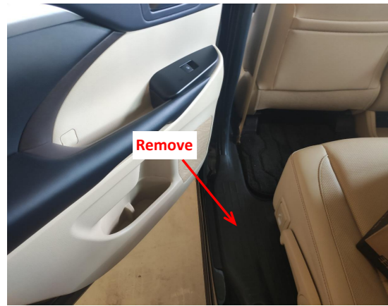
2. Remove the rear left side door sill panel.
