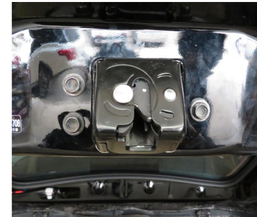
5. Remove the original latch and install the power latch.
