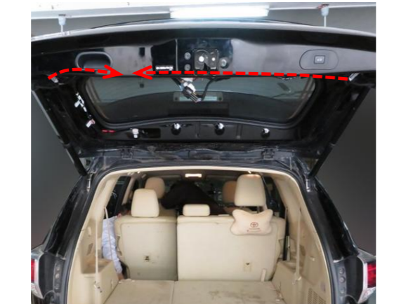
13. Route the strut wiring harnesses.
