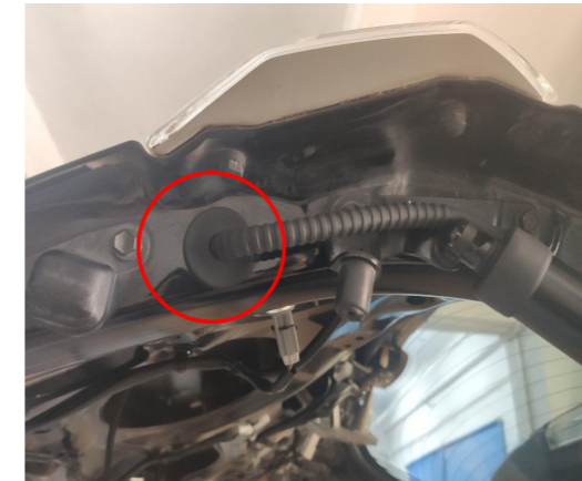
14. Plug the left and right holes with rubber plugs.
