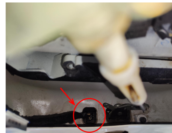
14. Connect the plugs of the lock signal harness to the indicated plug of the lock and its socket.
