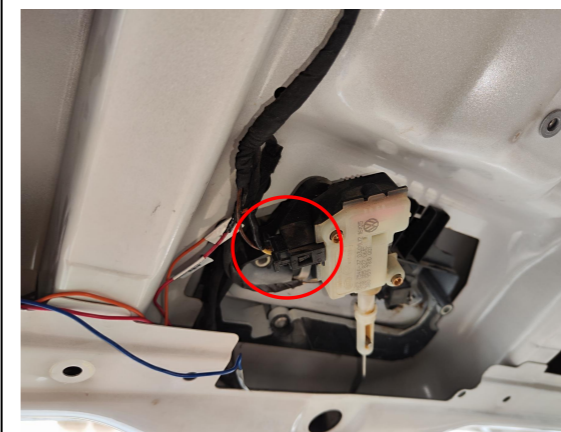
15. Connect the lock signal harness to the plugs of the lock motor.
