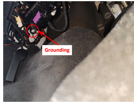
19. Ground at the left side of the pedals with the original ground wire connector.
