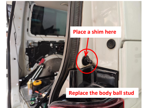
6. Replace the body ball stud and place a shim between the ball stud and vehicle body; both sides are the same.
