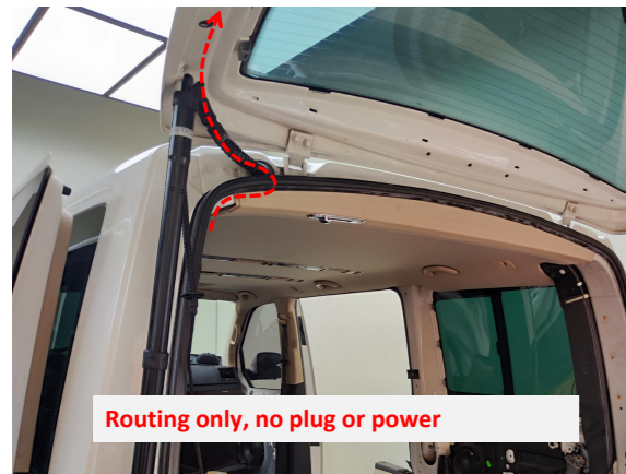
17. Thread power harness to the tailgate.
