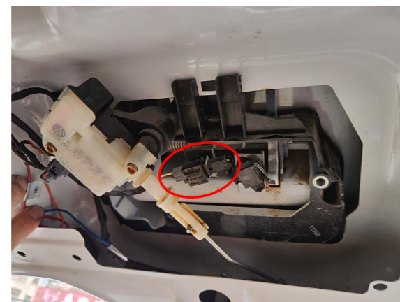
13. Connect the plugs of the lock signal harness to the plugs of original tailgate switch.
