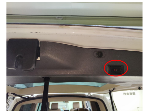
28. Reinstall all trim panels and install the added tailgate switch.
