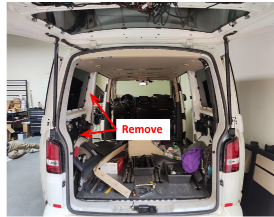
3. Remove the trim panels on the left side of the trunk to allow wiring harnesses to pass through.
