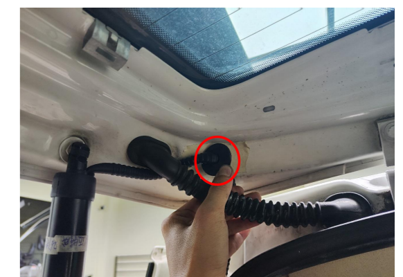
6. Replace the body ball stud and place a shim between the ball stud and vehicle body; both sides are the same.
