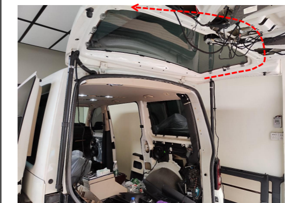
10. Route the strut wiring harnesses as indicated in the diagram.
