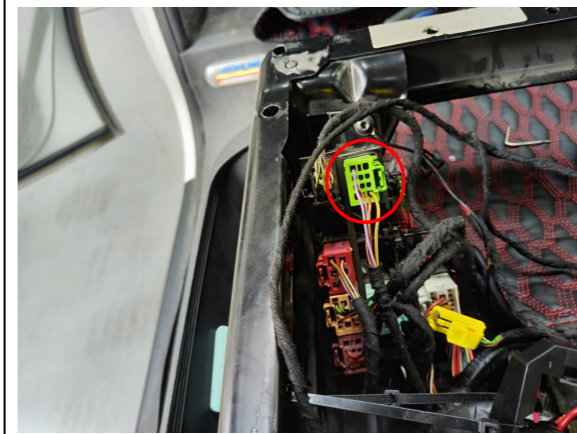
20. Connect the power harness to the indicated signal plug and its socket under the driver's seat.
