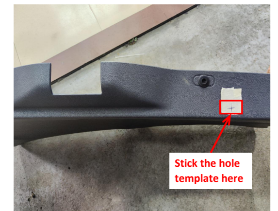
27. Open a hole at the indicated position for the added tailgate switch (as close as possible to the folded edge).
