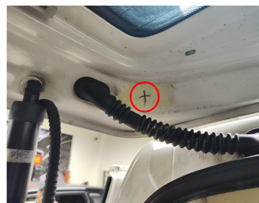
8. Drill a hole at the indicated position on the left side of the trunk with a \phi 21 mm drill bit to allow the wiring harness to pass through.
