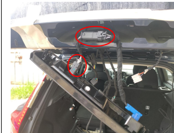
10. Connect the plugs of the lock signal harness to the lock latch, actuator and the added tailgate switch.
