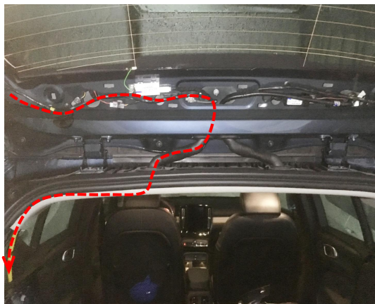
7. Route the signal harness to the left side of the trunk.
