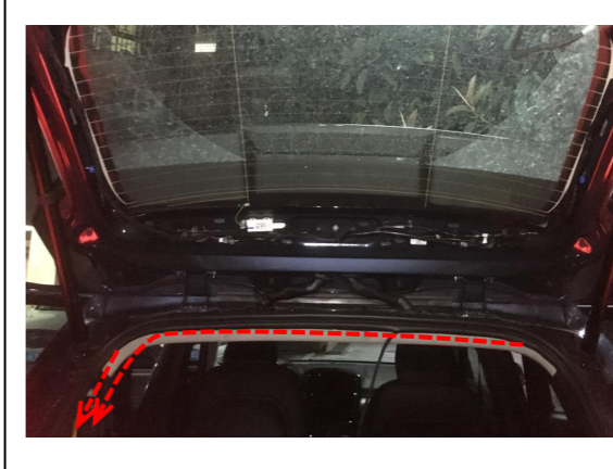
15. Route the strut wiring harnesses as indicated.
