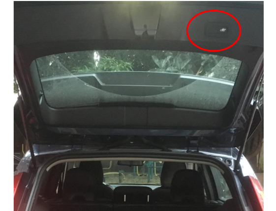
26. Reinstall all trim panels and fit the added tailgate switch in.
