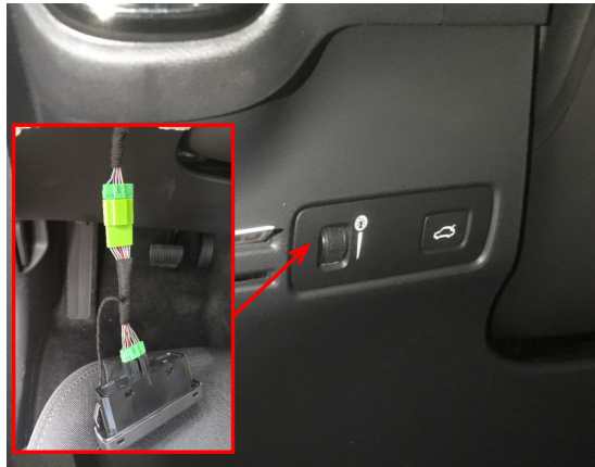
17. Connect the power harness to the plugs of the front tailgate switch.
