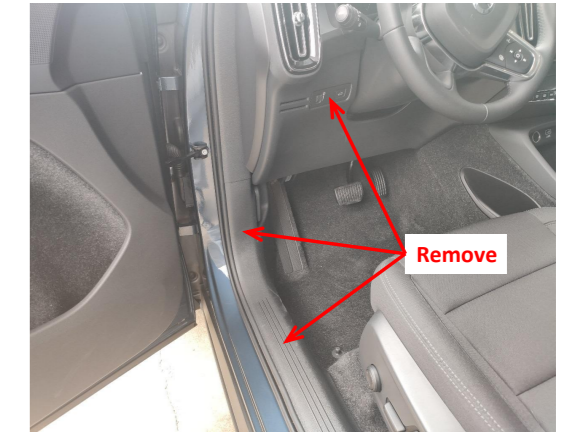
1. Remove the front left side door sill panels and the switch panel.
